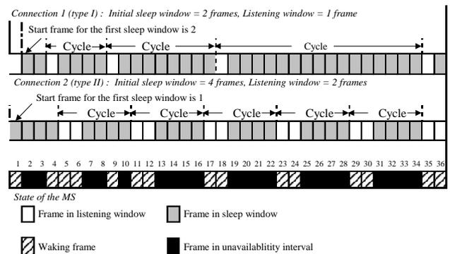
Fig. 2 Example of sleep mode operation
