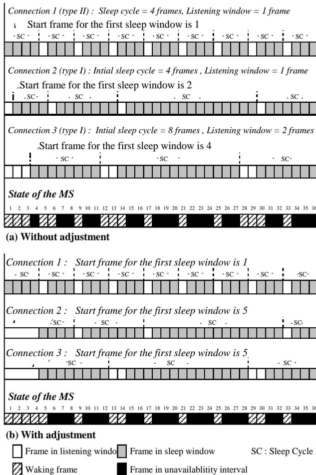
Fig. 4 Example of proposed power saving classes
