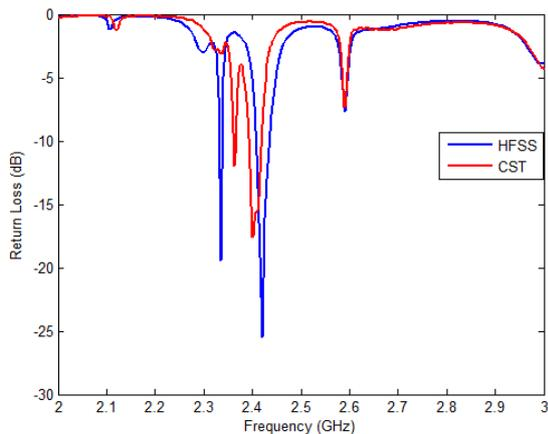
Fig.11: Return loss of the antenna linear array
