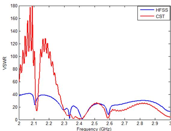
Fig.12: Voltage standing wave ratio of the antenna linear array
