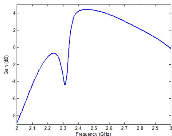
Fig.9: Gain of the single antenna element
