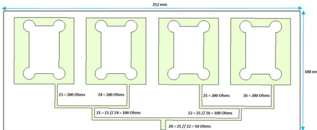
Fig.10: Geometry of the antenna linear array
