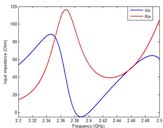
Fig.8: Input impedance of the single antenna element
