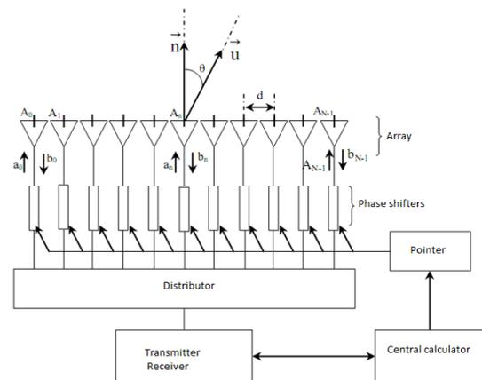
Fig.1 : General structure of a linear array
