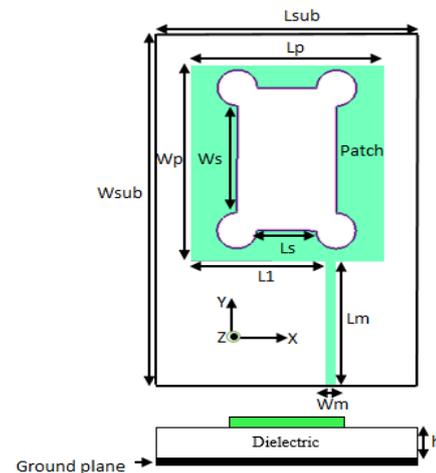
Fig.5: Geometry of the single antenna element proposed
