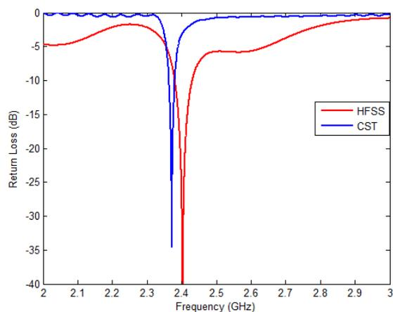
Fig.6: Return loss of the single antenna element
