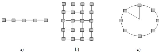
Fig.2 : Different geometric configurations of the arrays, linear (a), two-dimensional (b) and circular (c)
