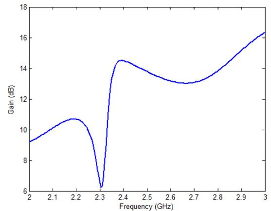
Fig.13: Gain of the antenna array
