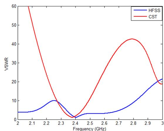
Fig.7: Voltage standing wave ratio of the single antenna element
