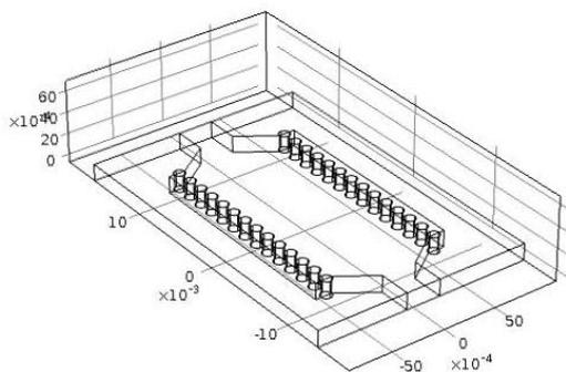
**Fig. 3** Structure of designed SIW
