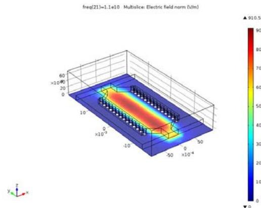
**Fig. 5(a)** Electric field for PCB substrate
