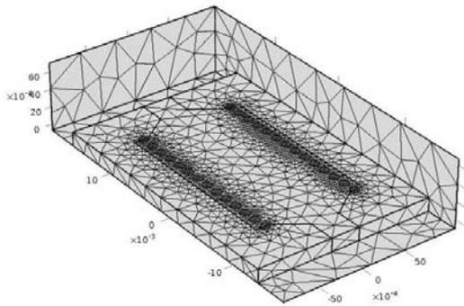
**Fig. 4** SIW structure while meshing is applied.
