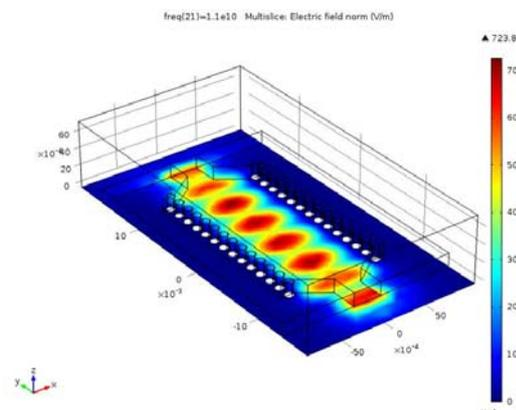
**Fig. 5(b)** Electric field for silicon substrate
