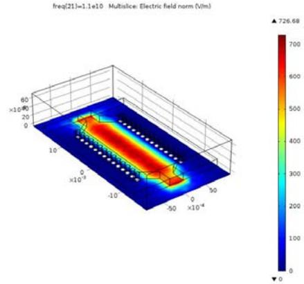
**Fig. 5(c)** Electric field for Mica substrate
