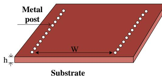
**Fig. 1** Schematic geometry of a SIW
