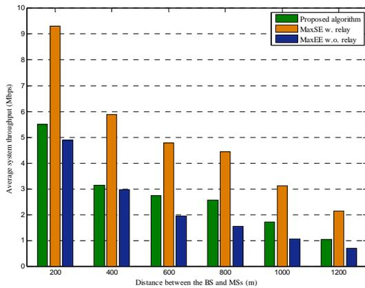
Figure 4 Average system throughput versus the distance between the BS and MSs (i.e.  $D_m$ )
