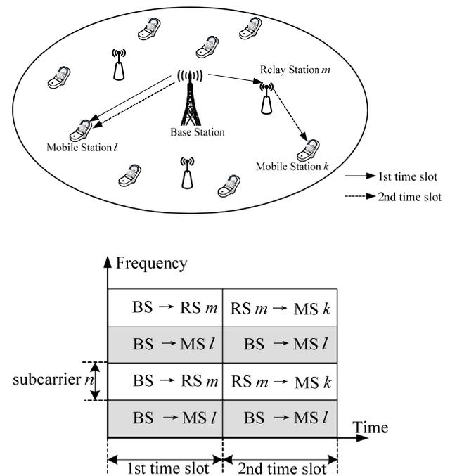
Figure 1 Example relay-enhanced OFDMA wireless cellular networks
