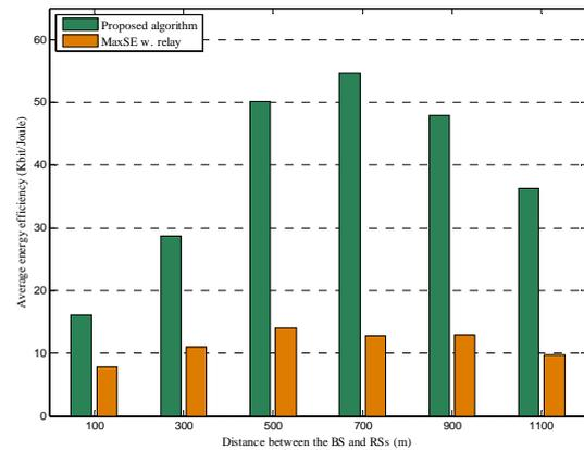
Figure 2 Average EE versus the distance between the BS and RSs (i.e.  $D_r$ )
