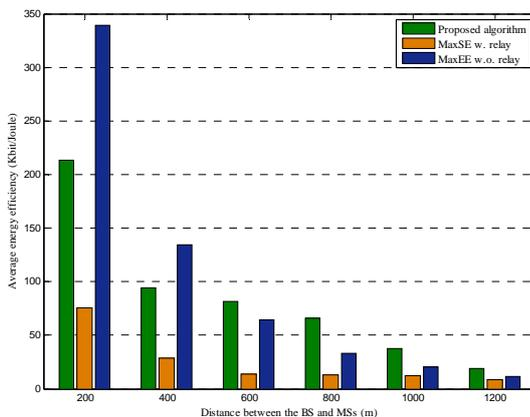
Figure 5 Average EE versus the distance between the BS and MSs (i.e.  $D_m$ )
