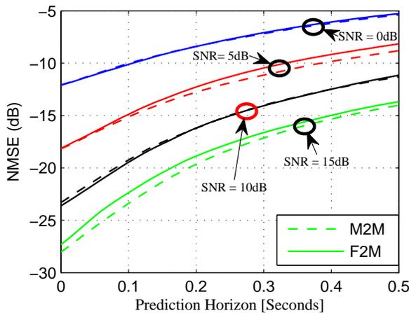
Figure 3: NMSE versus prediction horizon for M2M and F2M channel prediction at different SNR.
