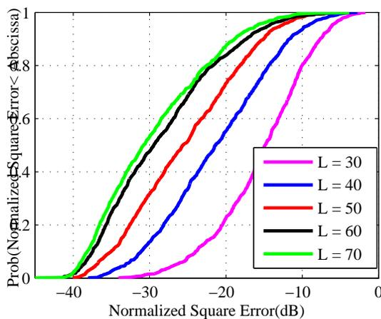
Figure 6: The CDF of prediction NSE for a prediction horizon of 100 ms at SNR = 10 dB with different number of samples in the training segment.
