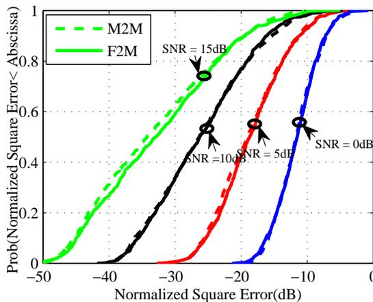
Figure 4: The CDF of NSE for a prediction horizon of 100 ms at SNR = 10 dB using 50 samples in the training segment.
