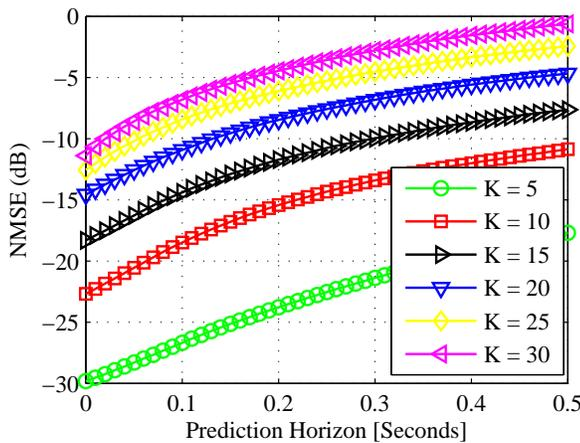
Figure 5: NMSE versus prediction horizon with different number of propagation paths at SNR = 10 dB.
