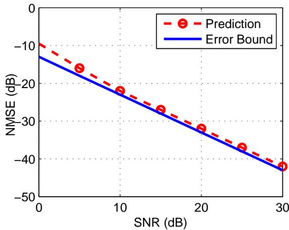
Figure 7: Prediction NMSE and error bound versus SNR for a prediction horizon of 50 ms with 100 samples in the observation segment.
