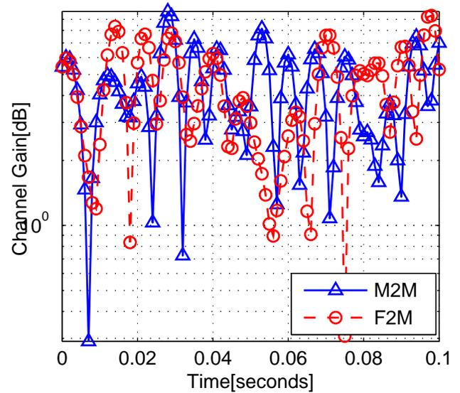
Figure 2: Amplitude of Mobile to Mobile (M2M) and Fixed to Mobile (F2M) Channel versus Time.
