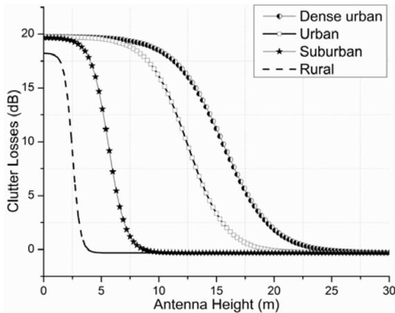
**Fig. 3** Clutter loss values as functions of antenna height for different environments
