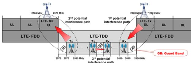
Fig. 2 Potential interferences in 2.6 GHz band
