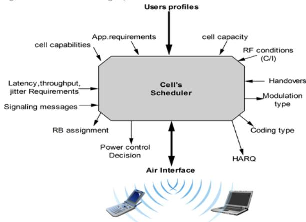
Fig. 4 Inputs and outputs of an LTE scheduler
