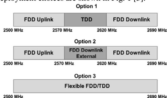
**Fig. 1** LTE deployment choices in 2.6 GHz band
