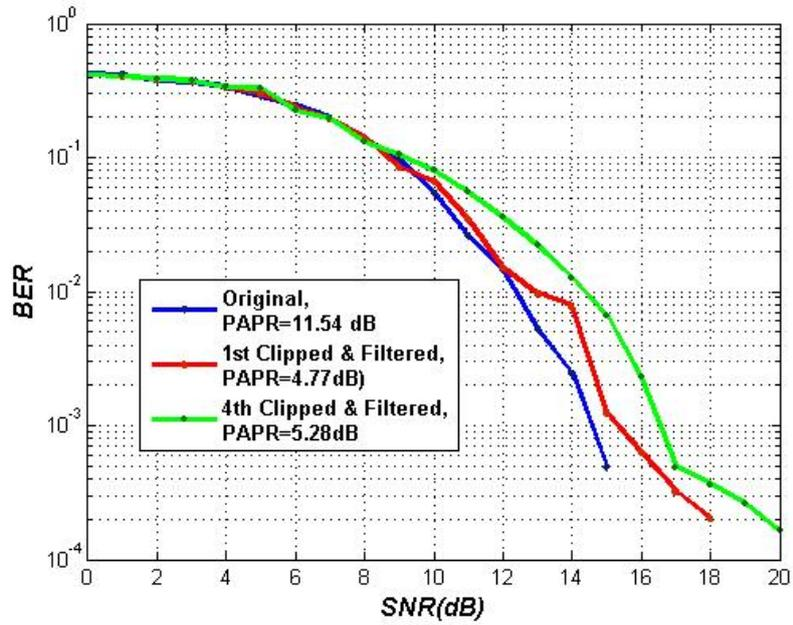
Figure 4: BER performances degrade after RCF for 16QAM 256 OFDM under AWGN channel. At 14 dB of  $E_b/N_o$ , BER increases slightly for 4<sup>th</sup> clipping and filtering
