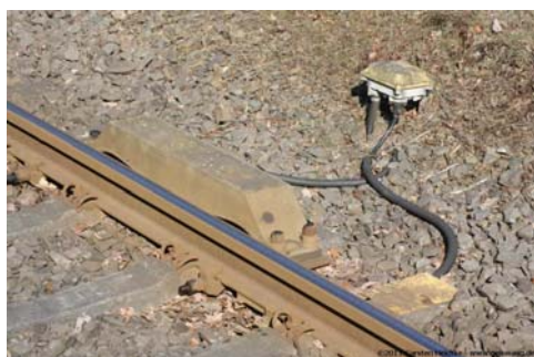
Fig. 2 INDUSI system – placement and cable connections [17]
