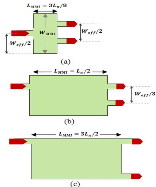
Fig.1 Schematic diagram of  $1 \times 2$  power splitter in (a) Symmetrical, (b) Paired, and (c) General Interference.
