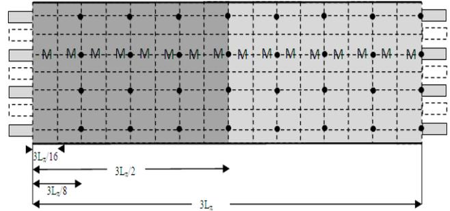
Fig. 6 Geometry of a  $4 \times 4$  MMI coupler
