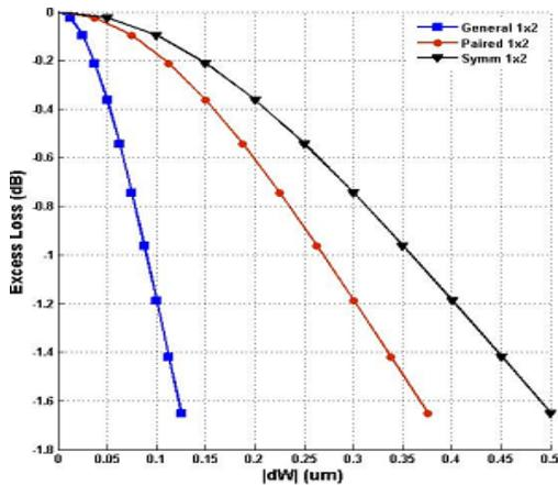
Fig.3 MMI Dimension tolerance W
