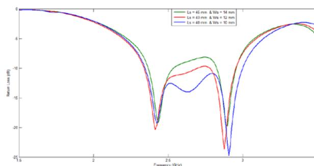
Fig.2: Return loss vs. frequency of the patch antenna
