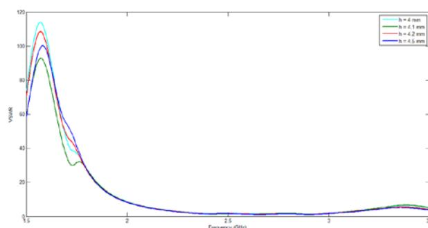
Fig.4: VSWR vs. frequency of the patch antenna
