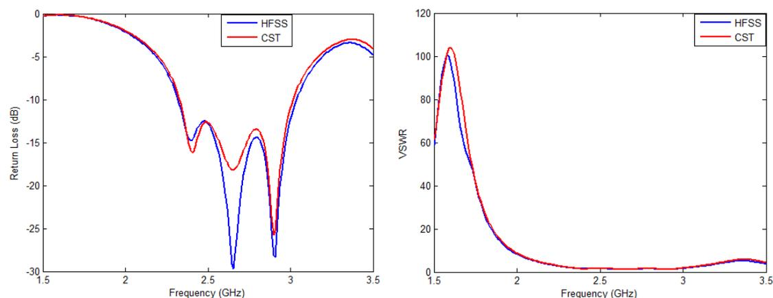
Fig.5: Comparison of simulation results in terms the reflection coefficient and voltage standing wave ratio using the simulators HFSS and CST
