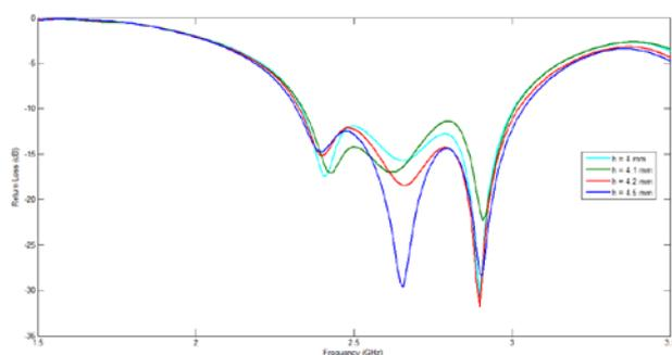
Fig.3: Return loss vs. frequency of the patch antenna
