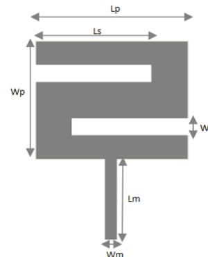
Fig.1: Geometry of a wide-band 2-shaped patch antenna
