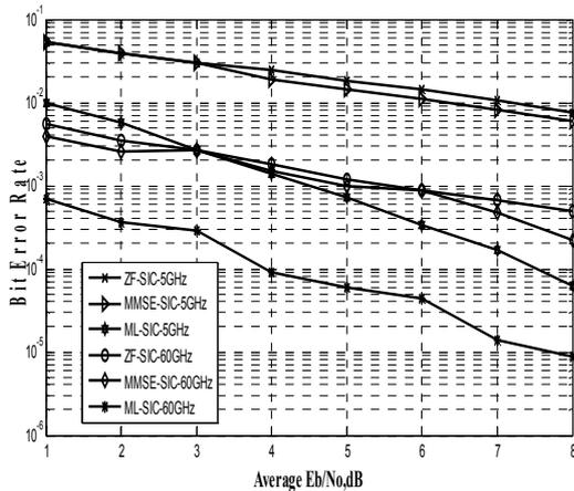
**Fig.13** Bit Error Rate of 4x4 system using TSV and Rayleigh channel models for indoor environment with transceiver separation of 3m.
