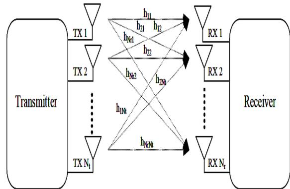
**Fig. 1** MIMO Transceiver
