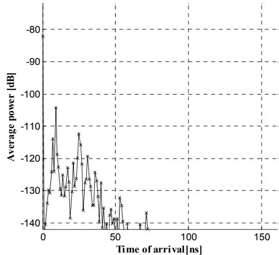
**Fig. 2** PDP of the TSV channel
