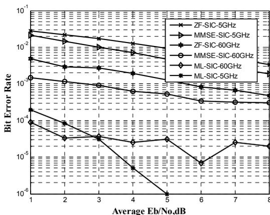
**Fig.14** Bit Error Rate of 8x8 system using TSV and Rayleigh channel models for indoor environment with transceiver separation of 3m.
