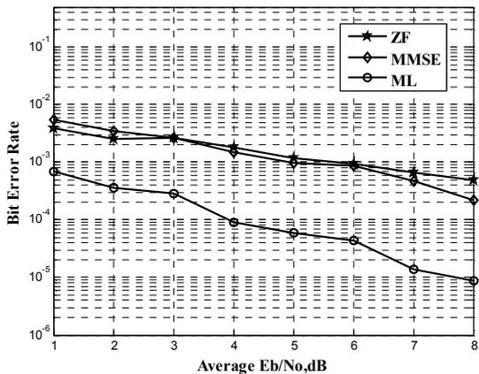
**Fig. 8** Comparison of BER for 4x4 MIMO system using ZFE, MMSE and ML technique.
