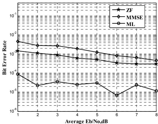
**Fig. 9** Comparison of BER for 8x8 MIMO system using ZFE, MMSE and ML technique.
