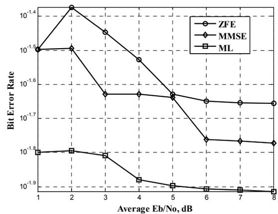
**Fig. 7** Comparison of BER for 2x2 MIMO system using ZFE, MMSE and ML technique.
