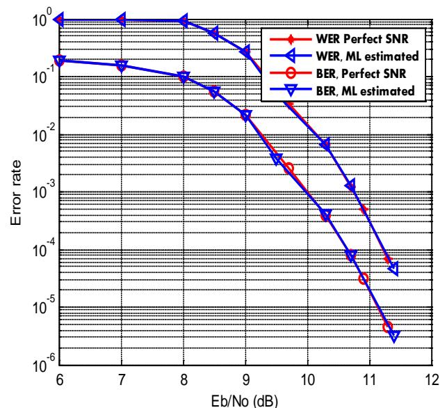
**Fig. 8** BER and WER of a rate-1/2 regular LDPC code with SNR perfectly known and estimated using ML estimation method.
