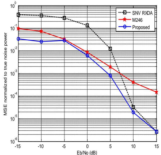
**Fig. 2** NMSE of the two proposed methods as compared to the conventional SNV RXDA method.
