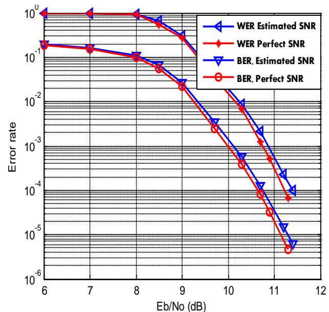
**Fig. 7** BER and WER of a rate-1/2 regular LDPC code with SNR perfectly known and estimated using the Higher-order statistics method.
