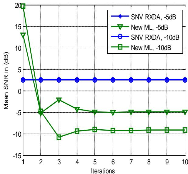
**Fig. 6** Mean estimated SNR vs. no. of iterations for ML estimation algorithm as compared to conventional SNV RXDA estimation [21] for negative SNRs.
