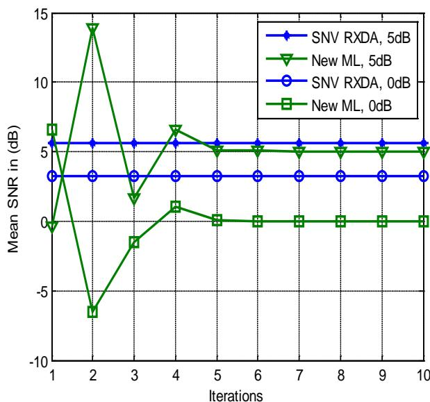
**Fig. 5** Mean estimated SNR vs. no. of iterations for ML estimation algorithm as compared to conventional SNV RXDA estimation [21].
