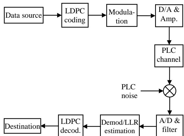
**Fig. 4** Simulation system arrangement
