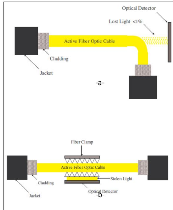
Fig.3: Optical Tapping Using Splitter and Coupler Method
