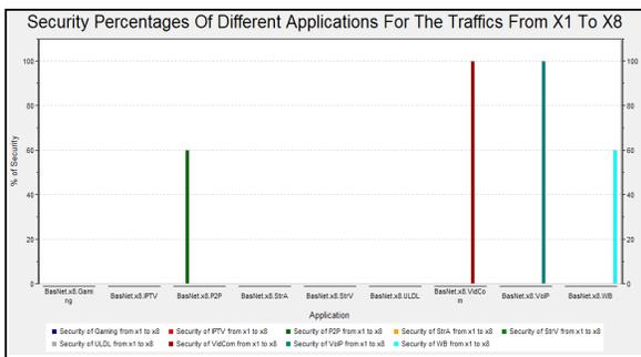
Fig.10: Security Percentages of Different Applications for the Traffics from X1 To X8
