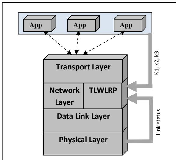
Fig.4: Internet Layered System with TLWLRP
