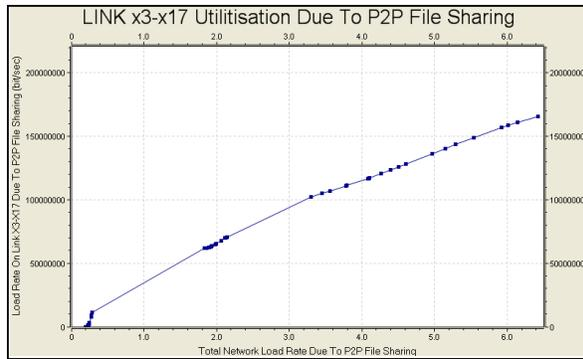
Fig.6: Link x3-x17 Utilisation Due To P2P File Sharing
