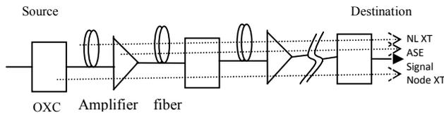
Fig. 1. Transmission path model used
