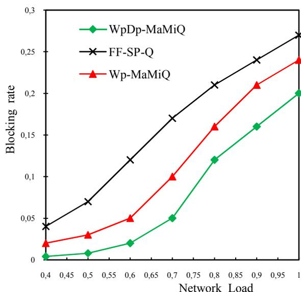
Fig.13.Blocking rate Vs Network Load for 20% protected demand for NFSNET
