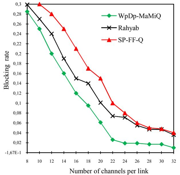
Fig.6. Call blocking rate Vs Number of channels per link (Load =70%) for 30% protected demand for DTNet
