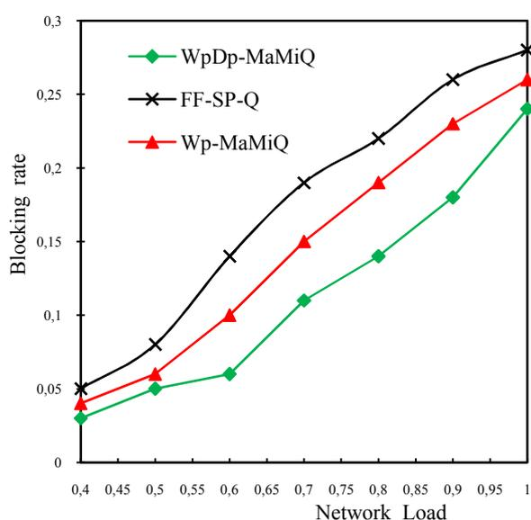
Fig.14.Blocking rate Vs Network Load for 30% protected demand for NFSNET
