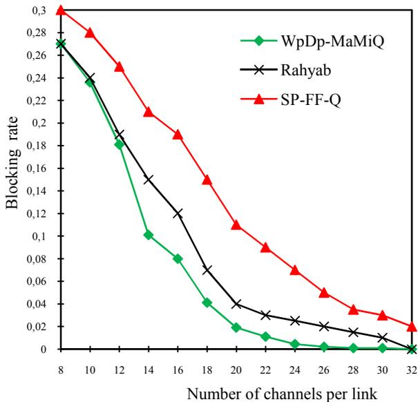
Fig.5. Call blocking rate Vs Number of channels per link (Load =70%) for 20% protected demand for DTNet
