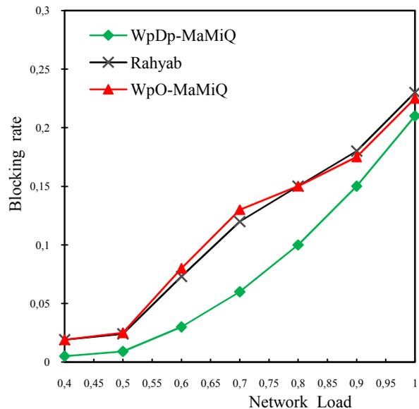
Fig.7. Blocking rate Vs Network Load for 20% protected demand for DTNet
