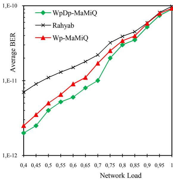
Fig.9. Average BER Vs Load for 20% protected demand for DTNet
