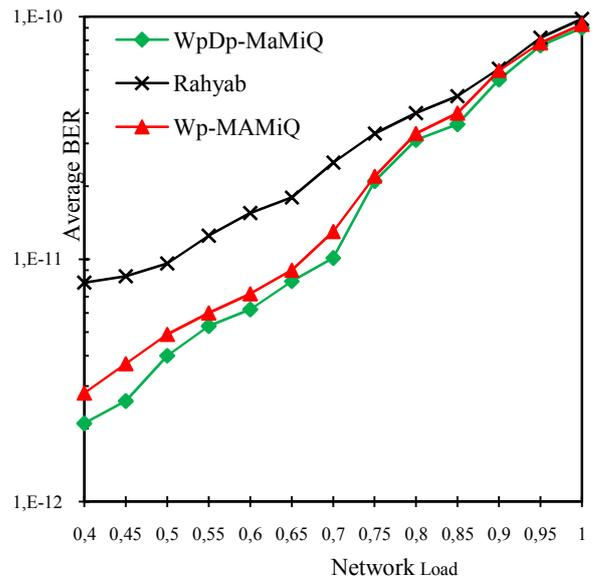
Fig.10. Average BER Vs Load for 30% protected demand for DTNet
