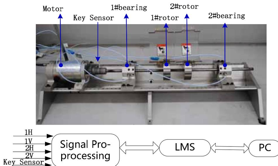
Fig. 6 Bently vibration system
