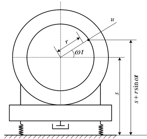
Fig. 3 Diagram of single freedom vibration system with single-disk rotor
