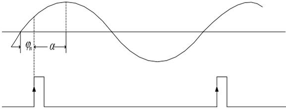
Fig. 2 Phase diagram of vibration signal triggered by key phase signal
