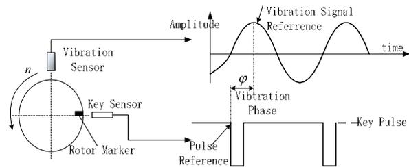
Fig. 1 The principle diagram of pulse method to measure the phase
