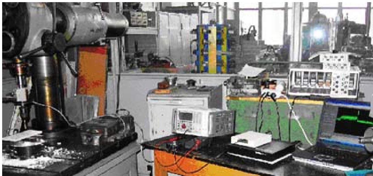
Fig. 2 Experimental stand - for force and torque study on machining holes
