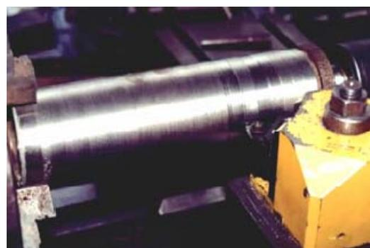
Fig 10 Turning sample in surface roughness experiments
