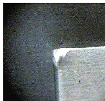
Fig. 8 Cutting tool VB wear
