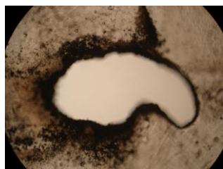
Fig. 15 Surface Damaged due to Electric stress 90kV/mm at 60 °C
