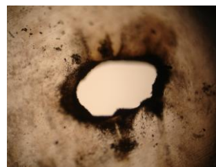
Fig. 17 Surface Damaged due to Electric stress 90kV/mm at 90 °C
