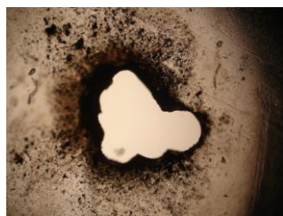
Fig. 14 Surface Damaged due to Electric stress 90 kV/mm at 23 °C
