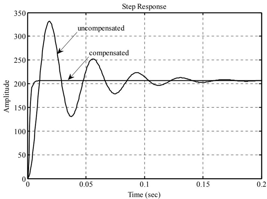
Fig. 10 Step responses of the head-stack.
