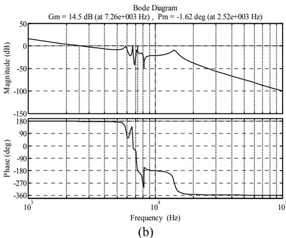
Fig. 2 Open-loop responses of the single-head: (a) time-domain, and (b) frequency-domain.
