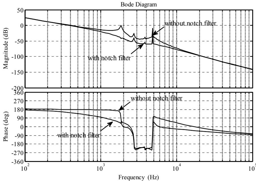
Fig. 6 Frequency responses of the head-stack without and with notch filters.
