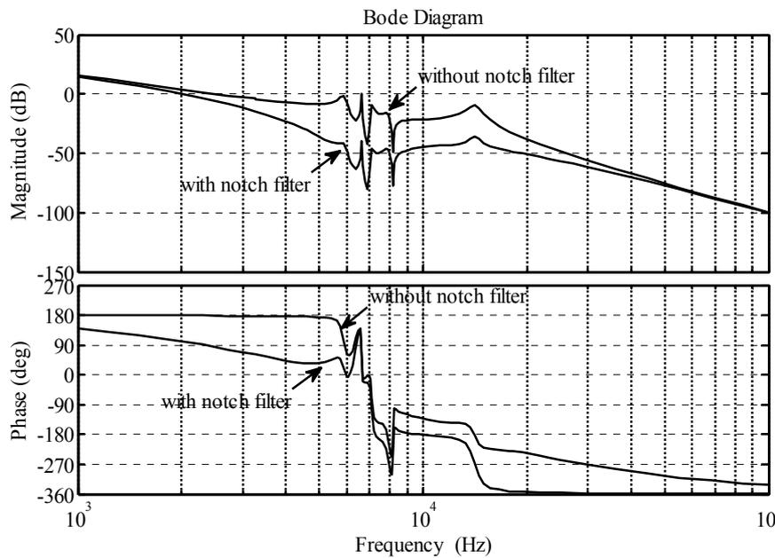
Fig. 5 Frequency responses of the single-head without and with notch filters.
