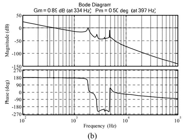
Fig. 3 Open-loop responses of the head-stack: (a) time-domain, and (b) frequency-domain.
