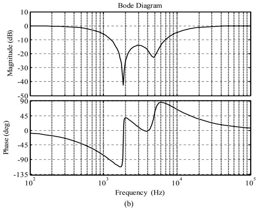
Fig. 4 Notch filter characteristics: (a) for single-head, and (b) for head-stack.
