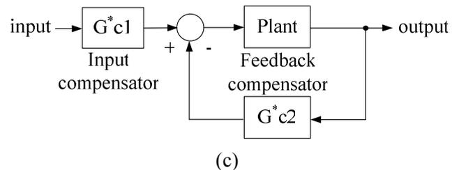
Fig. 7 System structures: (a) 1-DOF, (b) 2-DOF of type-I, and (c) 2-DOF of type-II.
