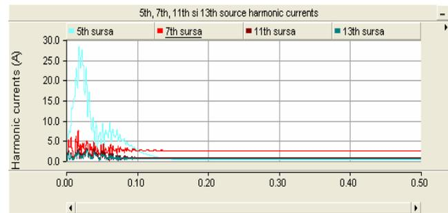
Fig.14a). Harmonic source currents using LC shunt passive filter (5th harmonic).
