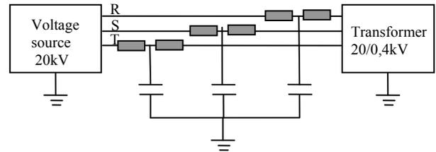
Fig.7. Low-pass passive filter.
