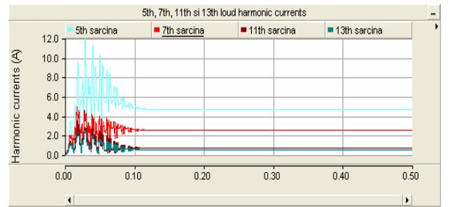
Fig.14b). Harmonic load currents using LC shunt passive filter (5th harmonic).
