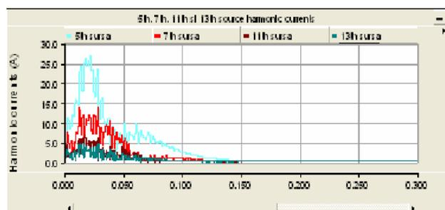
Fig.23a). Harmonic source currents for installation with all studied parallel passive filter.
