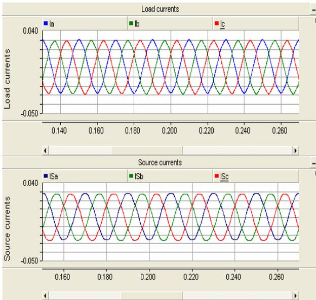
Fig.18. Source and load currents for installation using low-pass passive filter.
