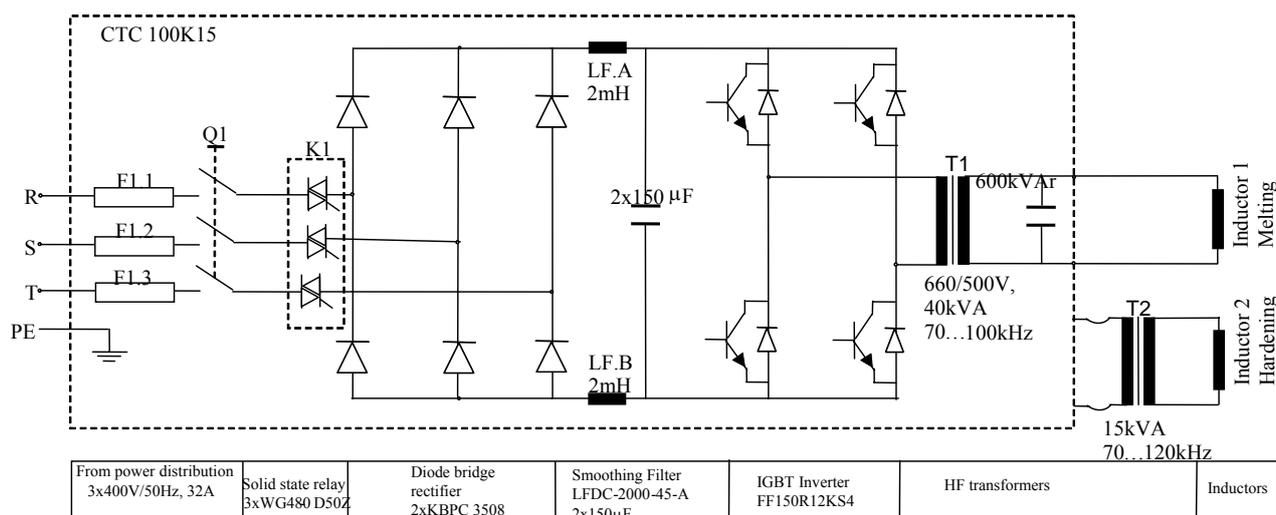
Fig.1. Melting/hardening electrothermal installation.
