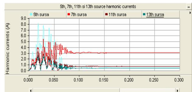
Fig.17a) Harmonic source currents for installation using series passive filter.
