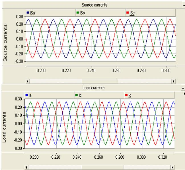
Fig.9. Source and load currents for nonfiltered installation.
