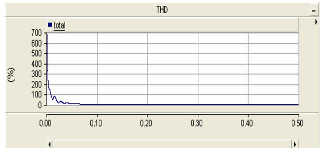
Fig.16. Total harmonic distortion in installation with series passive filter.
