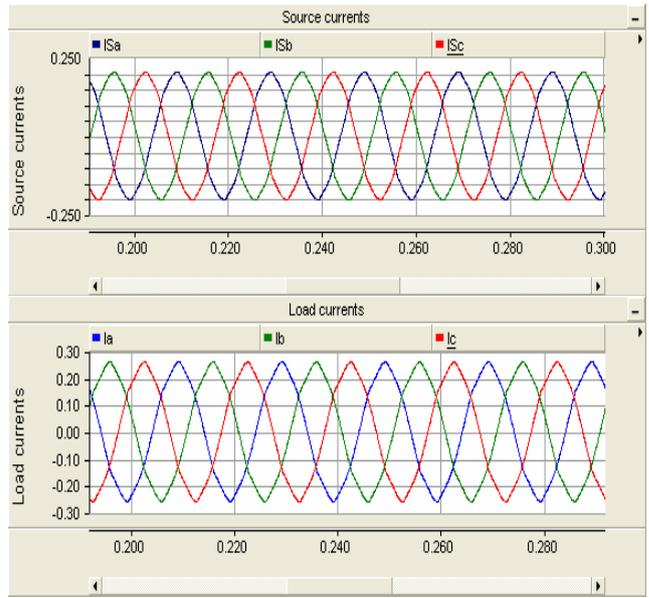
Fig.12. Source and load currents using LC shunt passive filter (5th harmonic).
