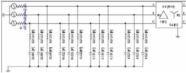
Fig.21. Parallel passive filter for all studied harmonics.
