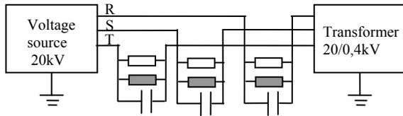
Fig.6. Series passive filter.
