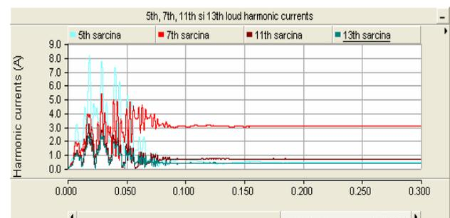
Fig.17b). Harmonic load currents for installation with series passive filter.
