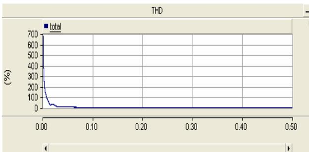
Fig.19. Total harmonic distortion in installation with low-pass passive filter.
