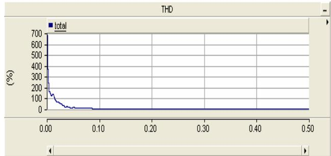
Fig.13. Total harmonic distortion using 5th harmonic filter.
