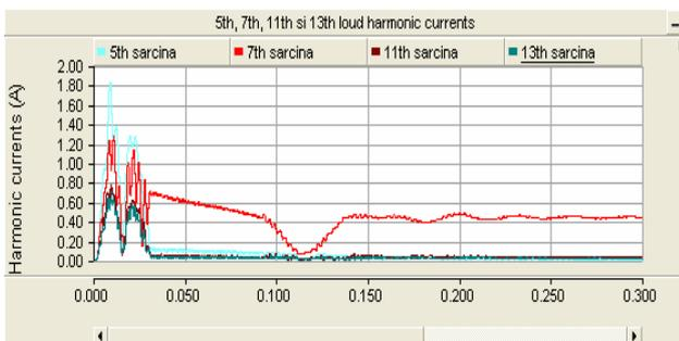
Fig.20b). Harmonic load currents for installation with low-pass passive filter.
