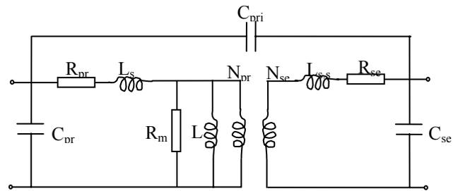
Fig.3. Equivalent scheme of the windings.
