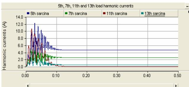
Fig.11b). Harmonic load currents in nonfiltered installation.
