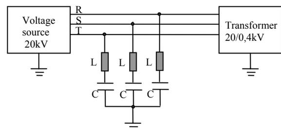
Fig.5. Parallel passive filter.
