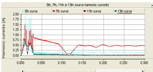
Fig.20a). Harmonic source currents for installation with low-pass passive filter.
