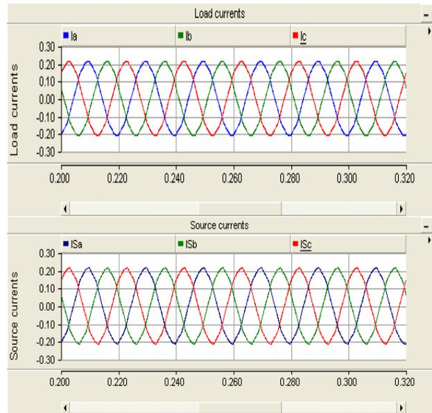
Fig.15. Source and load currents for installation using series passive filter.
