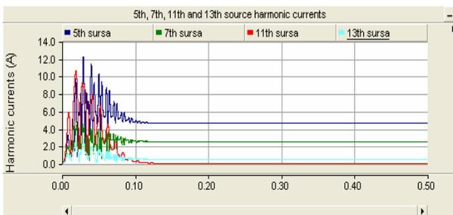
Fig.11a). Harmonic source currents in nonfiltered installation.
