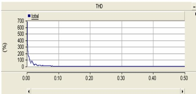
Fig.10. Total harmonic distortion in nonfiltered installation.
