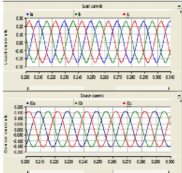
Fig.21. Source and load currents for installation using all studied parallel passive filter.
