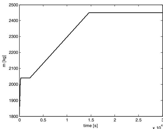
Fig. 22 The mass of reaction mixture – MPC1
