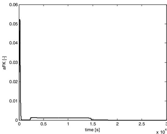
Fig. 21 The in-reactor chromium sludge concentration development – MPC1
