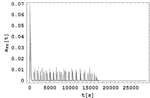
Fig. 10 The chromium sludge concentration development – two step control with penalization
