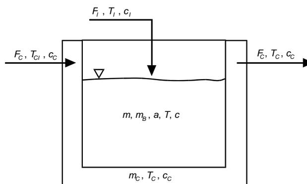
Fig. 2 Simplified scheme of exothermic chemical semi-batch reactor.
