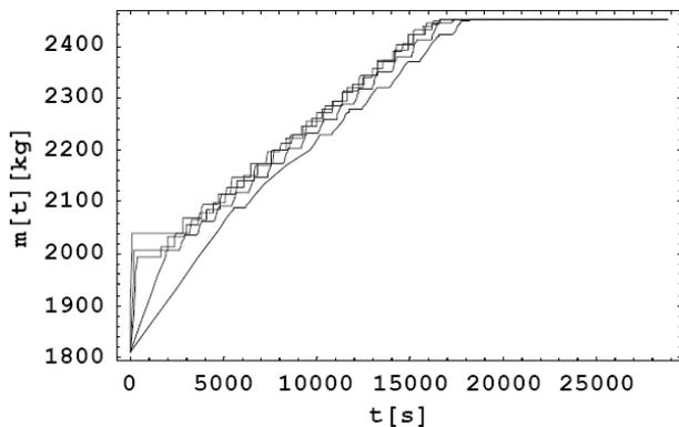
Fig. 3 The in-reactor mass development – two step control
