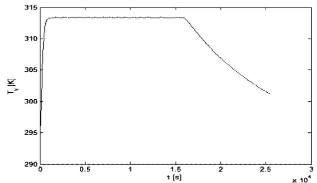
Fig. 15 The coolant temperature development – PID control
