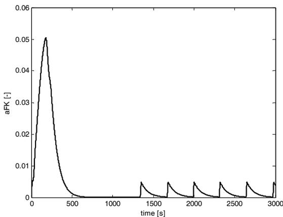
Fig. 25 The in-reactor chromium sludge concentration development – MPC2
