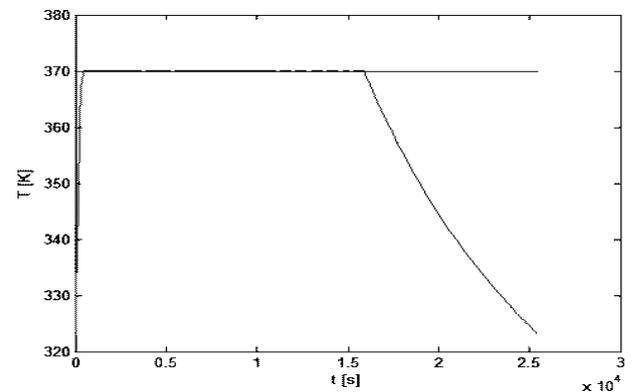
Fig. 14 The in-reactor temperature development – PID control
