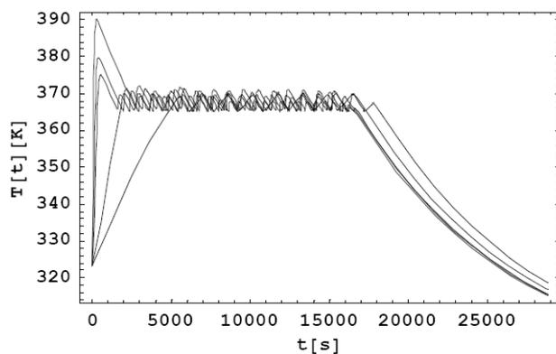
Fig. 4 The in-reactor temperature development – two step control
