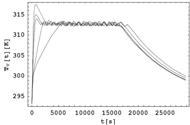
Fig. 5 The coolant temperature development – two step control
