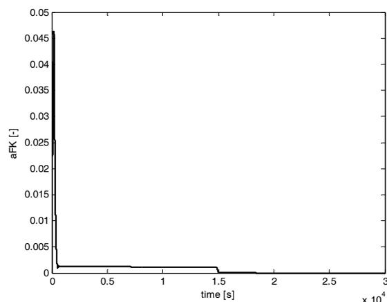
Fig. 29 The in-reactor chromium sludge concentration development – MPC3
