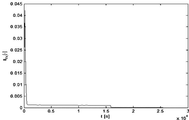
Fig. 16 The chromium sludge concentration development – PID control
