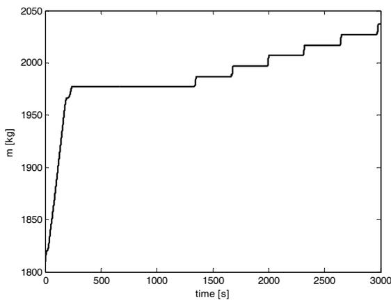
Fig. 26 The mass of reaction mixture – MPC2
