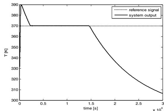
Fig. 19 The in-reactor temperature development – MPC1
