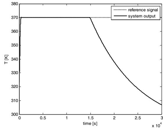
Fig. 27 The in-reactor temperature development – MPC3
