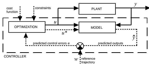
Fig. 17 The basic scheme of model predictive control
