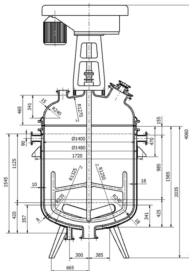
Fig. 1 Exothermic chemical semi-batch reactor.
