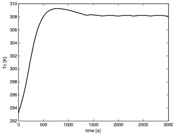
Fig. 24 The temperature in the cooling system – MPC2
