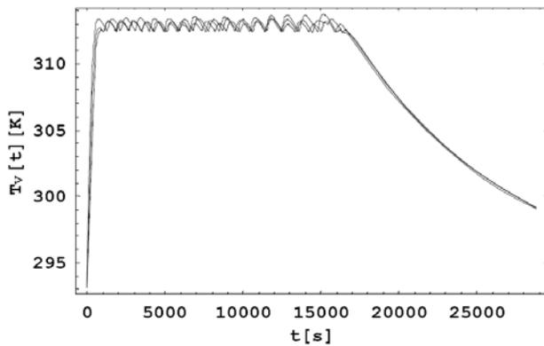
Fig. 9 The coolant temperature development – two step control with penalization
