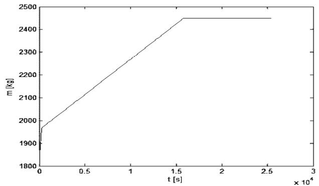
Fig. 13 The in-reactor mass development – PID control
