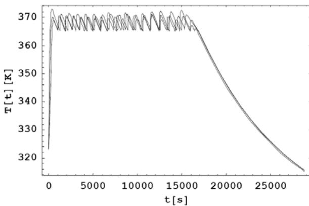
Fig. 8 The in-reactor temperature development – two step control with penalization
