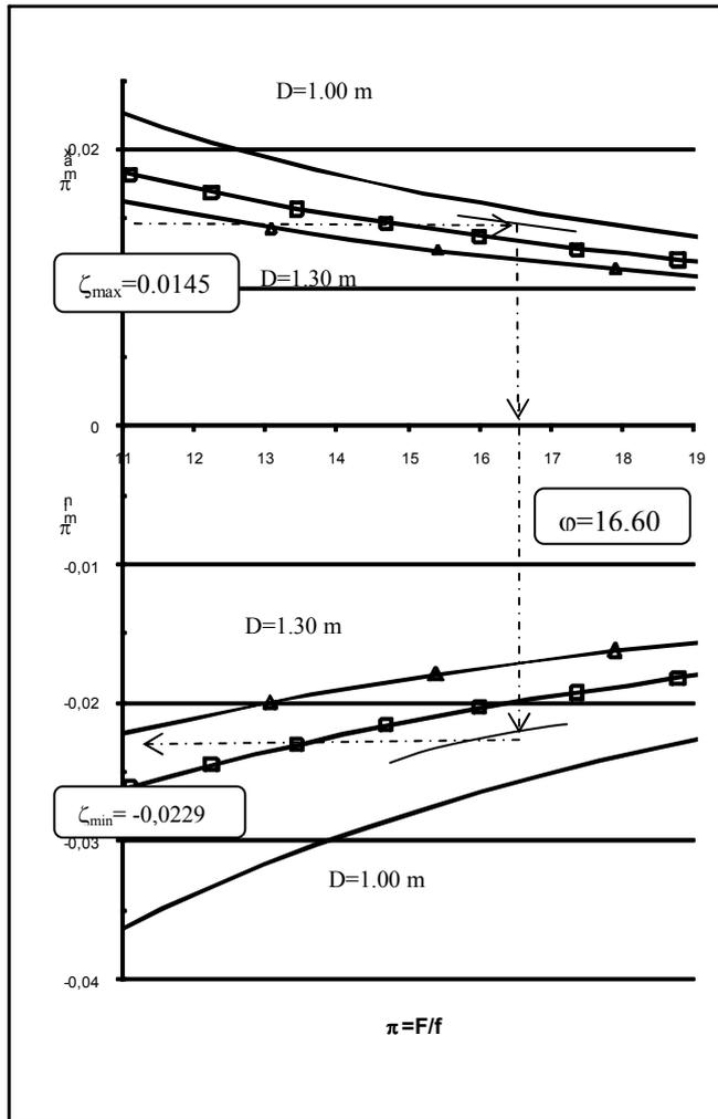
Fig.15. Graphical determination on the diagram for  $Q=3\text{m}^3/\text{s}$ ,  $L=500\text{m}$  and  $D=1.10\text{ m}$
