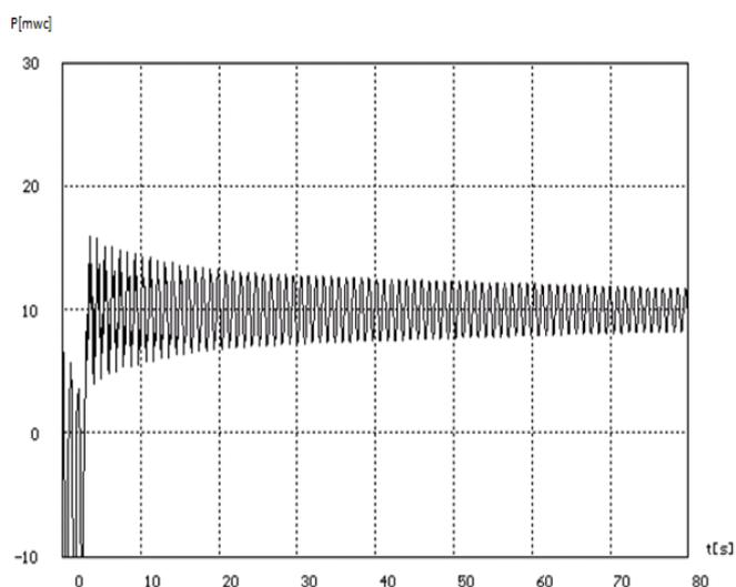
Fig.4 Pressure variation in node 1, for a duct diameter  $D=900$  mm
