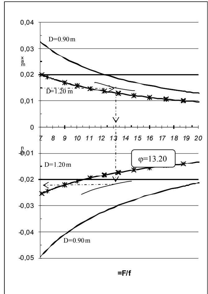
Fig.14. Graphical determination on the diagram for  $Q=2\text{m}^3/\text{s}$ ,  $L=500\text{m}$  and  $D=1.10 \text{ m}$
