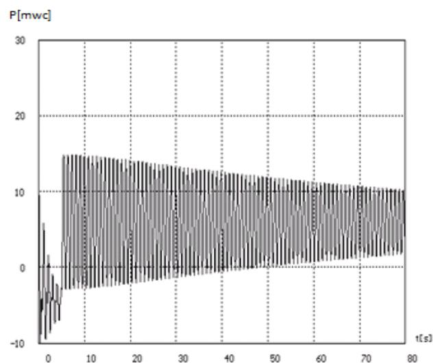
Fig.3 Pressure variation in node 5, for a duct diameter  $D=600$  mm
