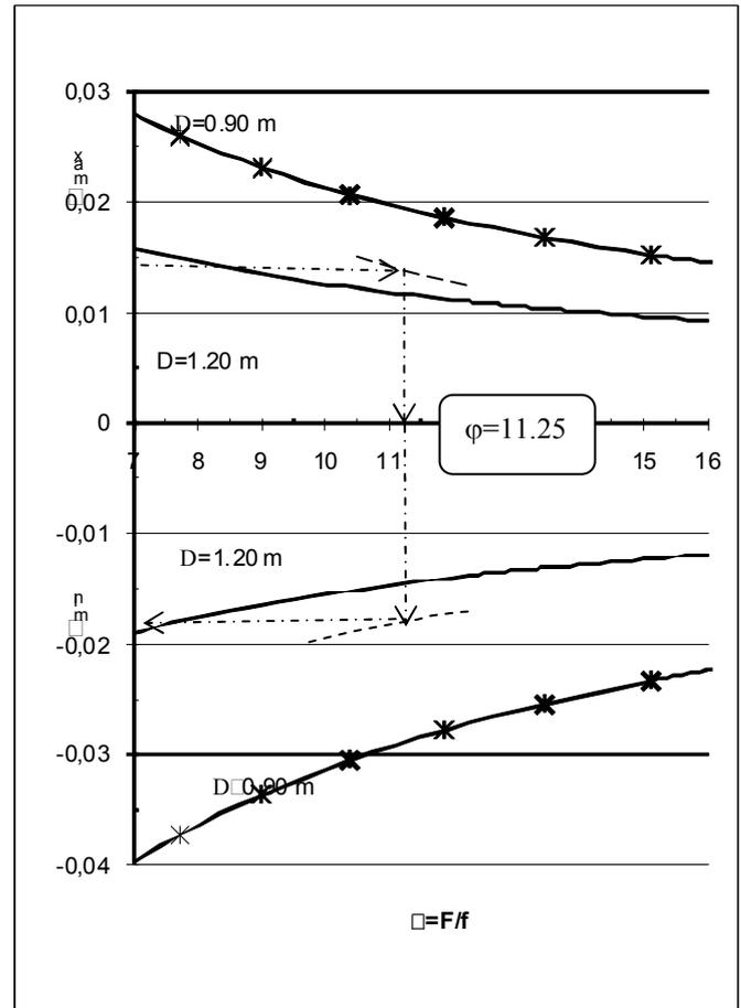
Fig.12. Graphical determination on the diagram for  $Q=2\text{m}^3/\text{s}$ ,  $L=250\text{m}$  and  $D=1.10 \text{ m}$
