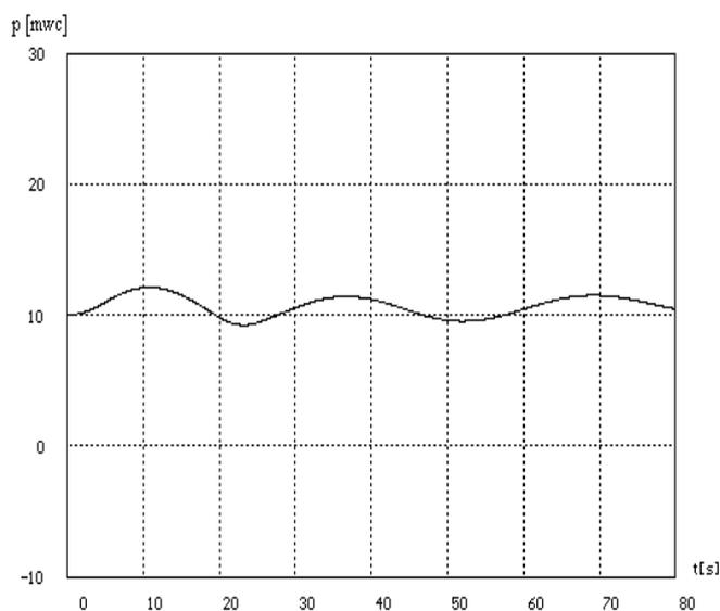
Fig.7 Water level inside the surge tank, in the case of 3 pumps discharging on a 900 mm pipeline. The pumps start one by one. Surge tank diameter  $D_{ST}=1000\text{mm}$ .
