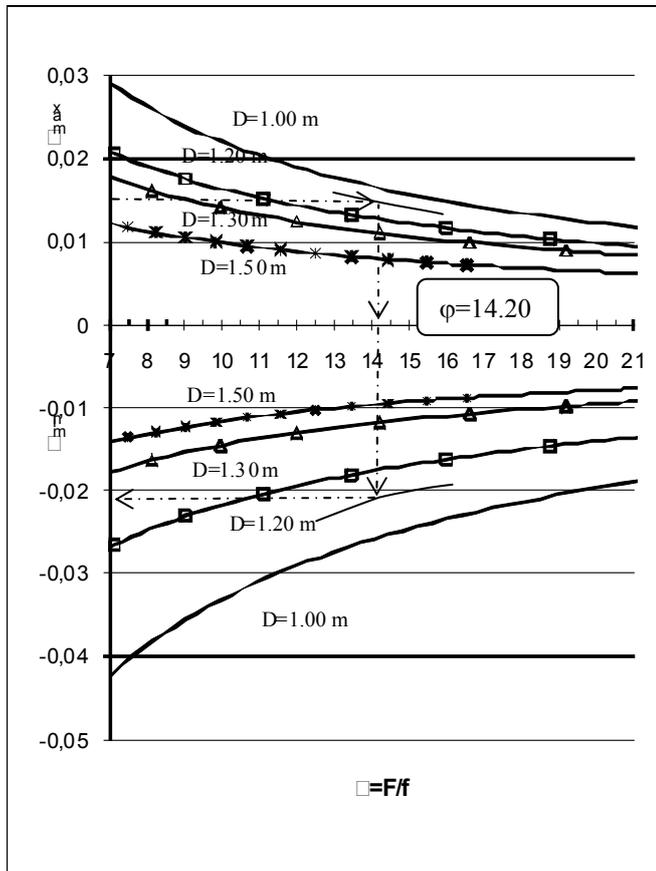
Fig.13. Graphical determination on the diagram for  $Q=3\text{m}^3/\text{s}$ ,  $L=250\text{m}$  and  $D=1.10 \text{ m}$
