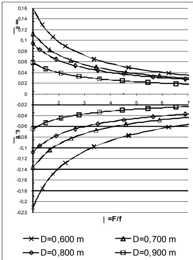
Fig.10. General diagram for surge tank dimensioning, for  $Q=1m^3/s$ ,  $L=250m$  and  $1<\varphi<7$
