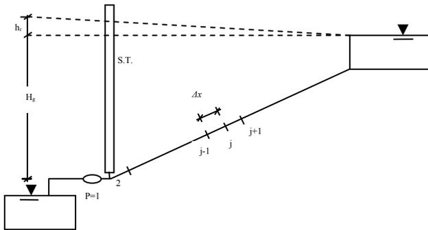
Fig.1 Pumping installation equipped with surge tank
