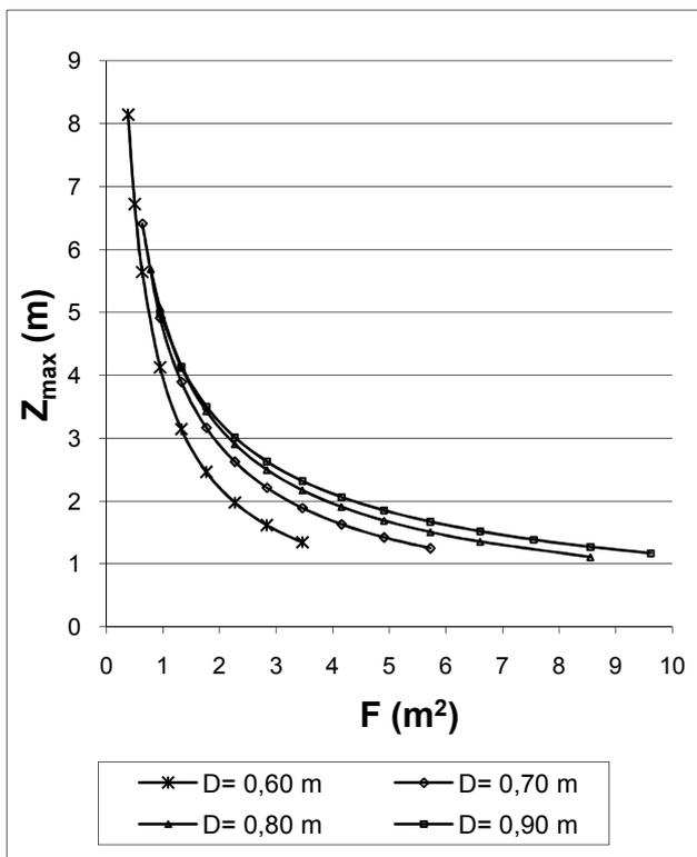
Fig.8. Maximal jump of the water level as a function of the surge tank cross section area
