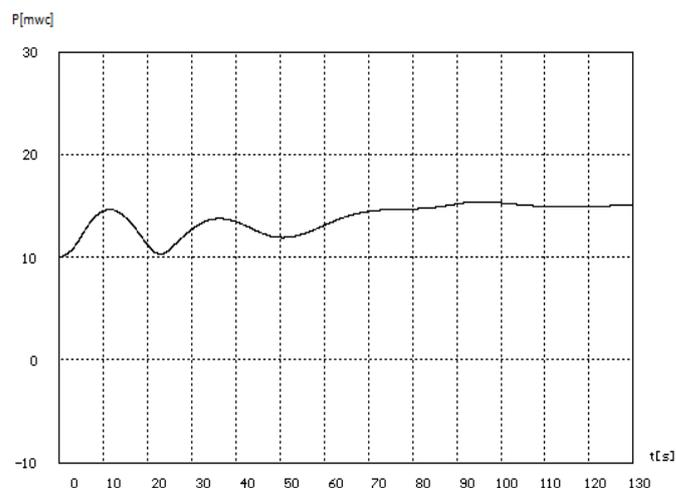
Fig.6 Water level inside the surge tank, in the case of 3 pumps discharging on a 600 mm pipeline. The pumps start one by one. Surge tank diameter  $D_{ST}=700$ mm.
