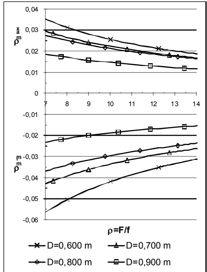
Fig.11. General diagram for surge tank dimensioning, for  $Q=1m^3/s$ ,  $L=250m$  and  $7<\varphi<14$
