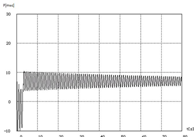
Fig.5 Pressure variation in node 4, for a duct diameter  $D=900$  mm
