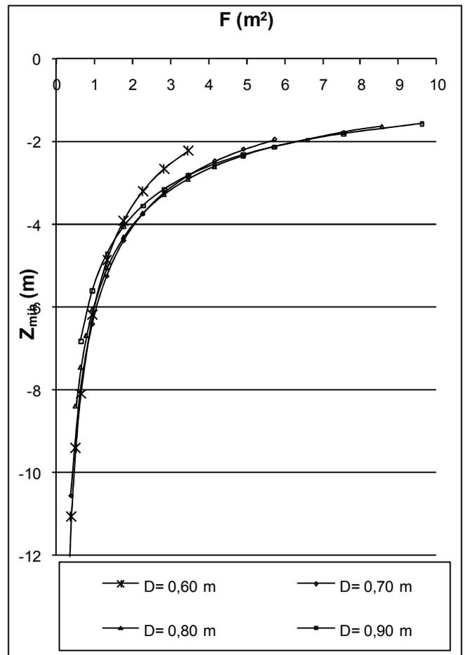
Fig.9. Minimal jump of the water level as a function of the surge tank cross section area
