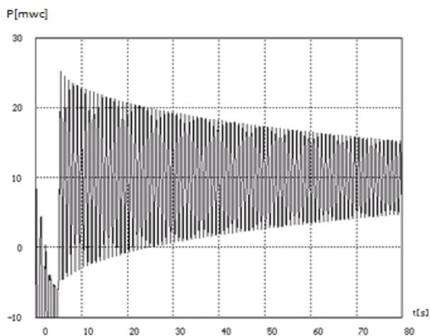
Fig.2 Pressure variation in node 1, for a duct diameter  $D=600$  mm
