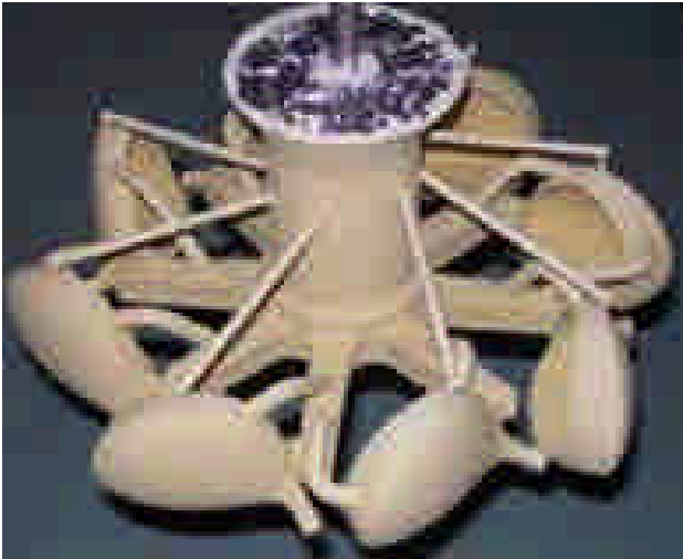
Fig.8 Coating forms the shell mould
