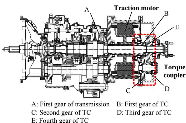
Fig. 4 Configuration of the T-EM
