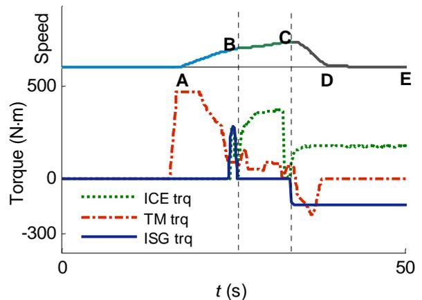
Fig. 17 Representative operation of the bus
