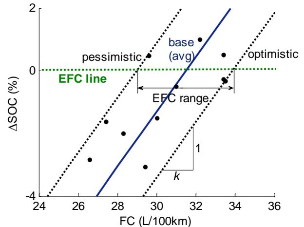
Fig. 19 Fuel consumptions vs. SOC intervals for the bus
