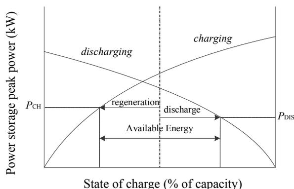
Fig. 13 Power capacity vs. SOC
