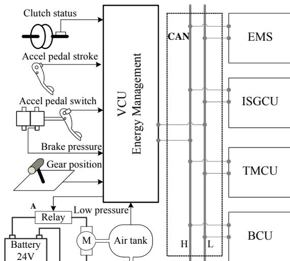
Fig. 8 Control network of SWB6116HEV
