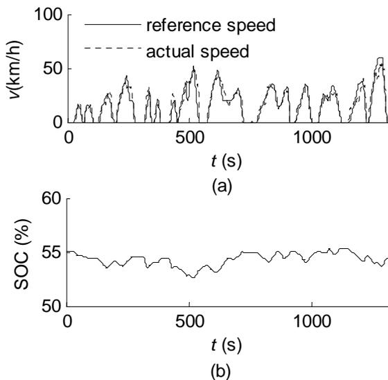
Fig. 18 Test case under CTBCDC: (a) reference and actual speed; (b) transient SOC.
