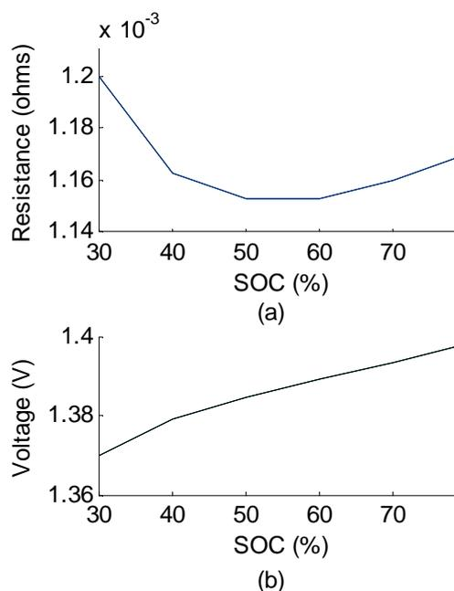
Fig. 14 Characteristic parameters of battery cells: (a) resistance; (b) open circuit voltage.
