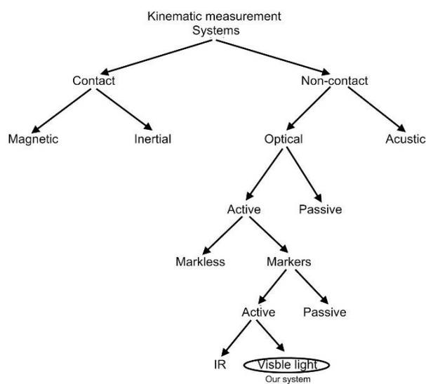
Fig. 1, Classification of kinematic measurement systems
