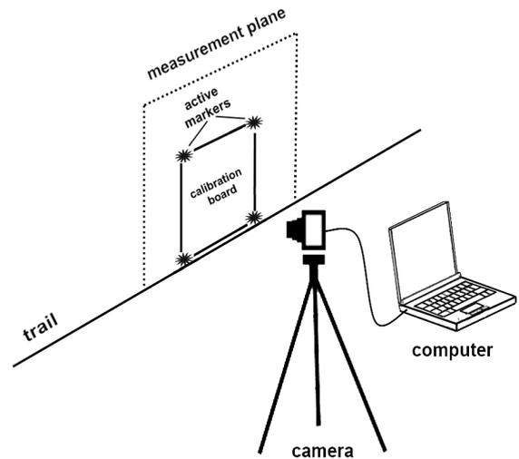
Fig. 3, Camera calibration setup
