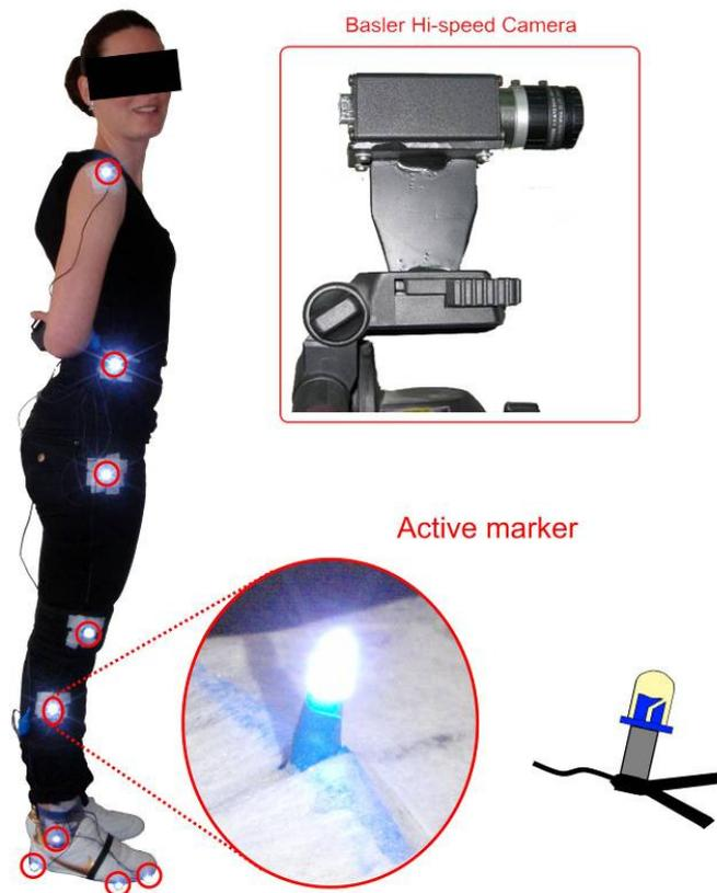
Fig. 2, Subject with attached active markers (left), fast industrial camera Basler 602fc (top) and enlarged active marker (bottom)
