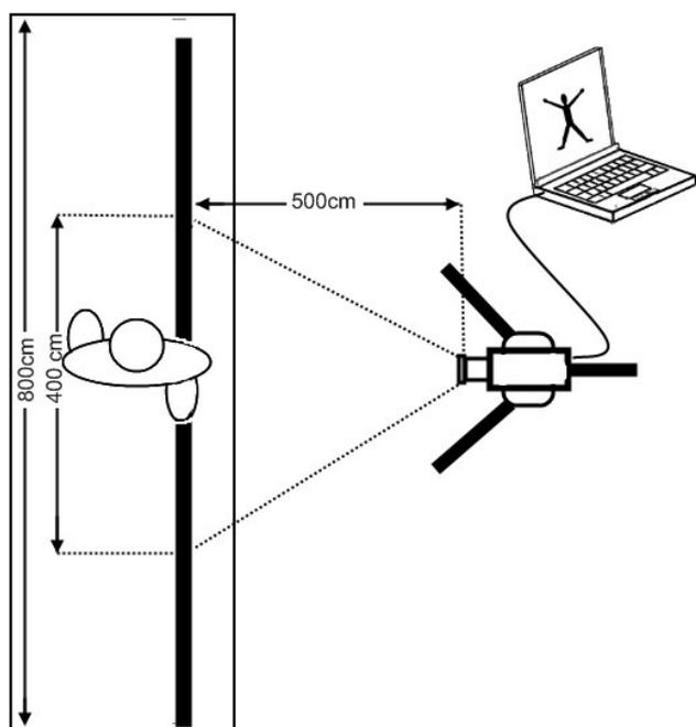
Fig. 5, Setup top-view, subject is walking following the line defining measurement plane
