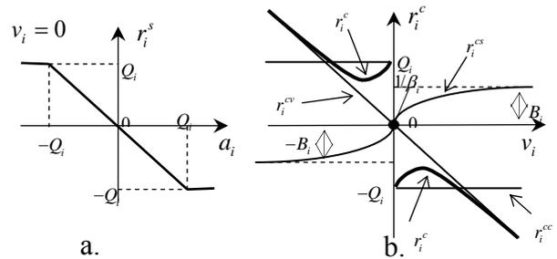
Fig.2, Static and cinematic components of a scalar friction reaction.
