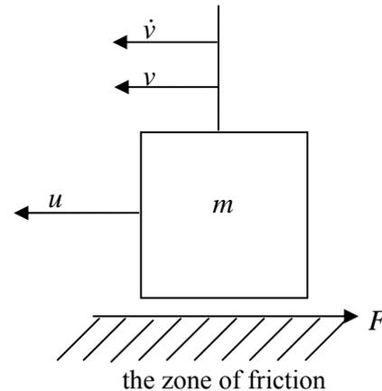
Fig.3, A simple mechanical system with friction
