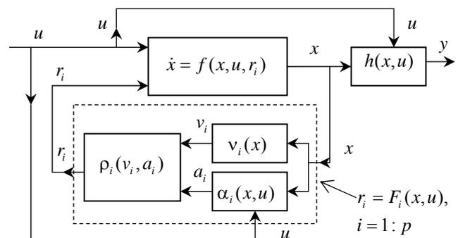
Fig.1, The feedback structure of a GFDS with SFM.
