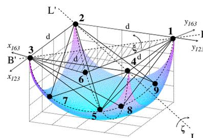
Fig.3. Nine-element USBL array
