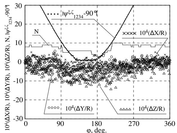
Fig.6. Variation of the relative errors of the object coordinates, number of the elemental USBL systems N that are used for calculation of coordinate means and modulus of the latitude angle to the transponder (object) relatively the USBL<sub>1234</sub> plane; R=100m; Z=40 m;  $\xi=-20^\circ$ ;  $\zeta=10^\circ$ .
