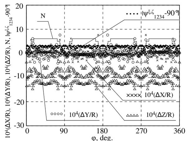
Fig.4. Variation of the relative errors of the object coordinates, number of the elemental USBL systems  $N$  that are used for calculation of coordinate means and modulus of the latitude angle to the transponder (object) relative to the USBL<sub>1234</sub> plane;  $R=100\text{m}$ ;  $Z=5\text{ m}$ ;  $\xi=0^\circ$ ;  $\zeta=0^\circ$ .
