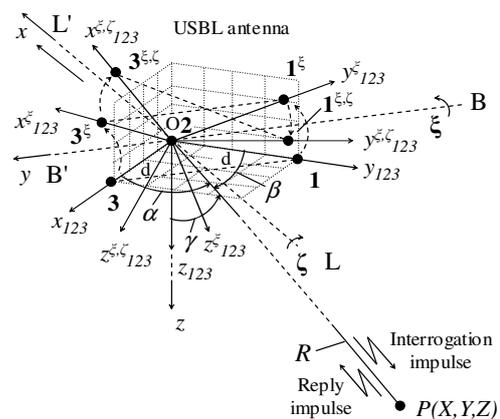
Fig.1. Geometry of the three-element USBL receiving array and the carrier longitudinal and lateral axes.
