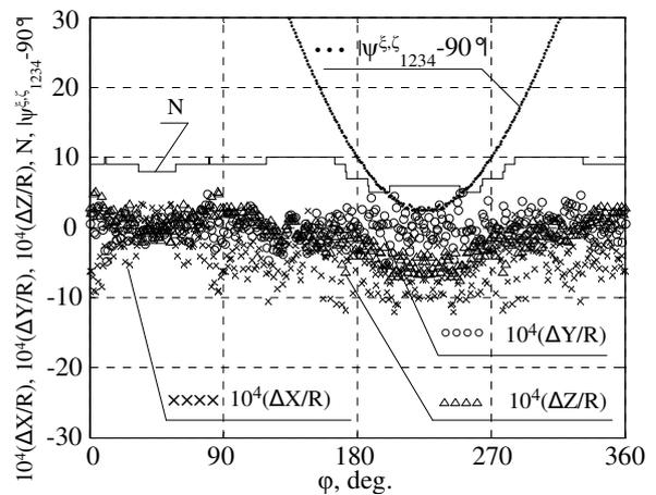
Fig.8. Variation of the relative errors of the object coordinates, number of the elemental USBL systems  $N$  that are used for calculation of coordinate means and modulus of the latitude angle to the transponder (object) relatively the  $USBL_{1234}$  plane;  $R=100\text{m}$ ;  $Z=150\text{ m}$ ;  $\xi = -40^\circ$ ;  $\zeta = -40^\circ$ .
