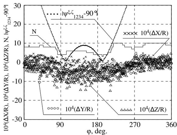
Fig.7. Variation of the relative errors of the object coordinates, number of the elemental USBL systems  $N$  that are used for calculation of coordinate means and modulus of the latitude angle to the transponder (object) relatively the  $USBL_{1234}$  plane;  $R=100\text{m}$ ;  $Z=50\text{ m}$ ;  $\xi = -30^\circ$ ;  $\zeta = 20^\circ$ .
