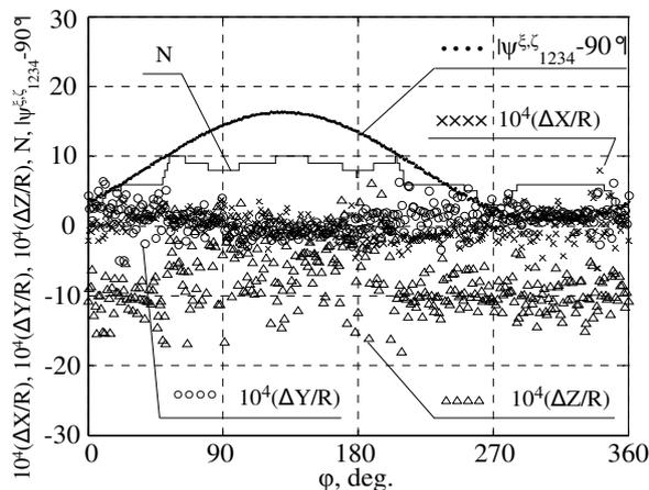
Fig.5. Variation of the relative errors of the object coordinates, number of the elemental USBL systems N that are used for calculation of coordinate means and modulus of the latitude angle to the transponder (object) relatively the USBL<sub>1234</sub> plane; R=100m; Z=15 m;  $\xi=5^\circ$ ;  $\zeta=-6^\circ$ .
