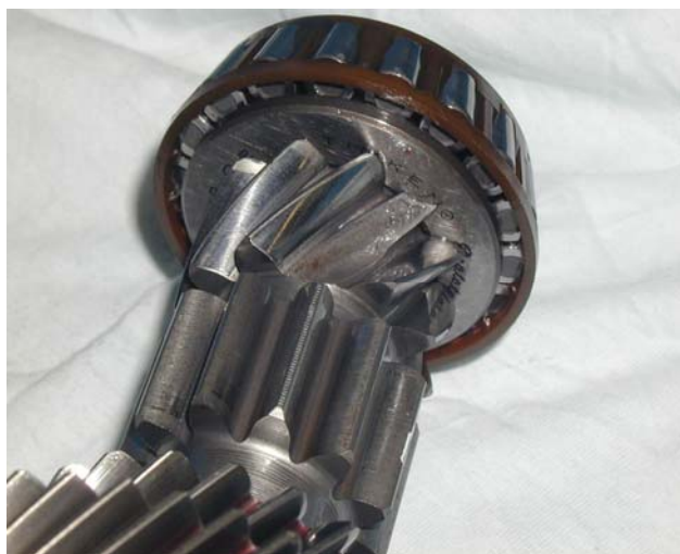
Fig.25 – Teeth condition following the first gear crack
