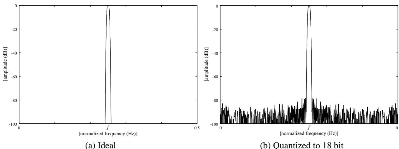
Figure 8: Frequency characteristics of the filter designed by proposed method
