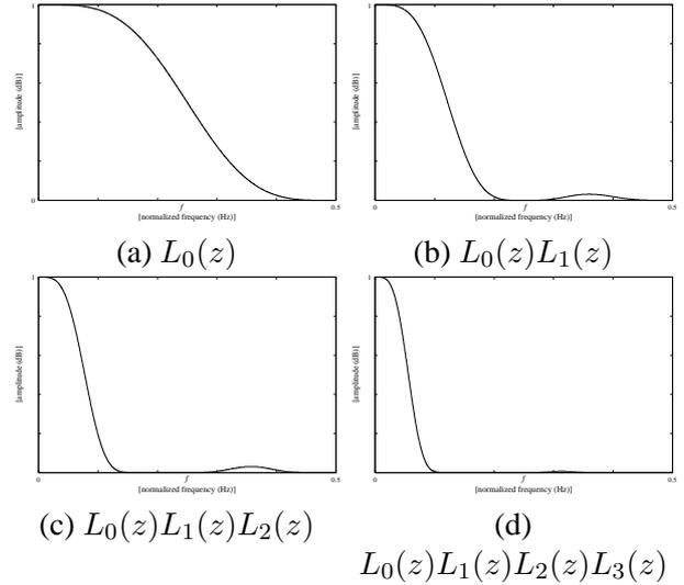
Figure 6: Connecting scaled filters
