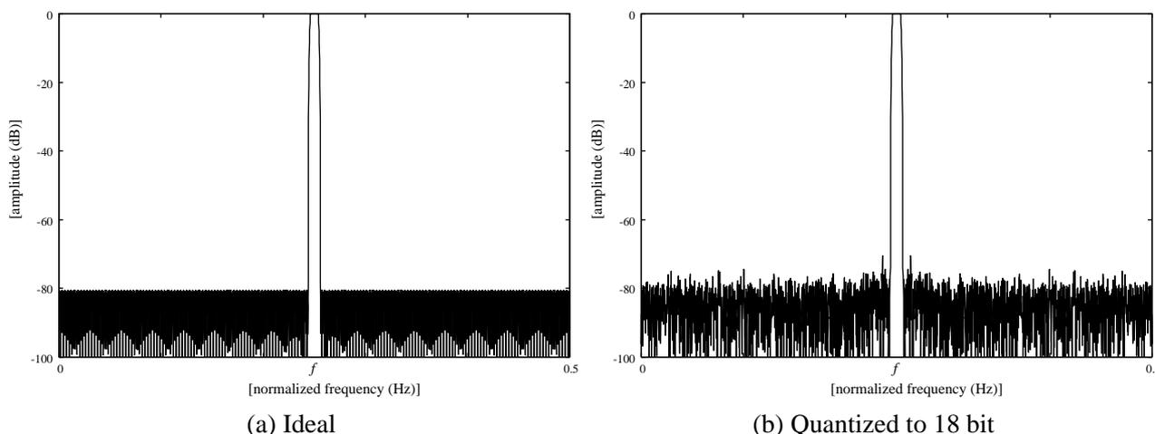
Figure 7: Frequency characteristics of the filter designed by Remez method
