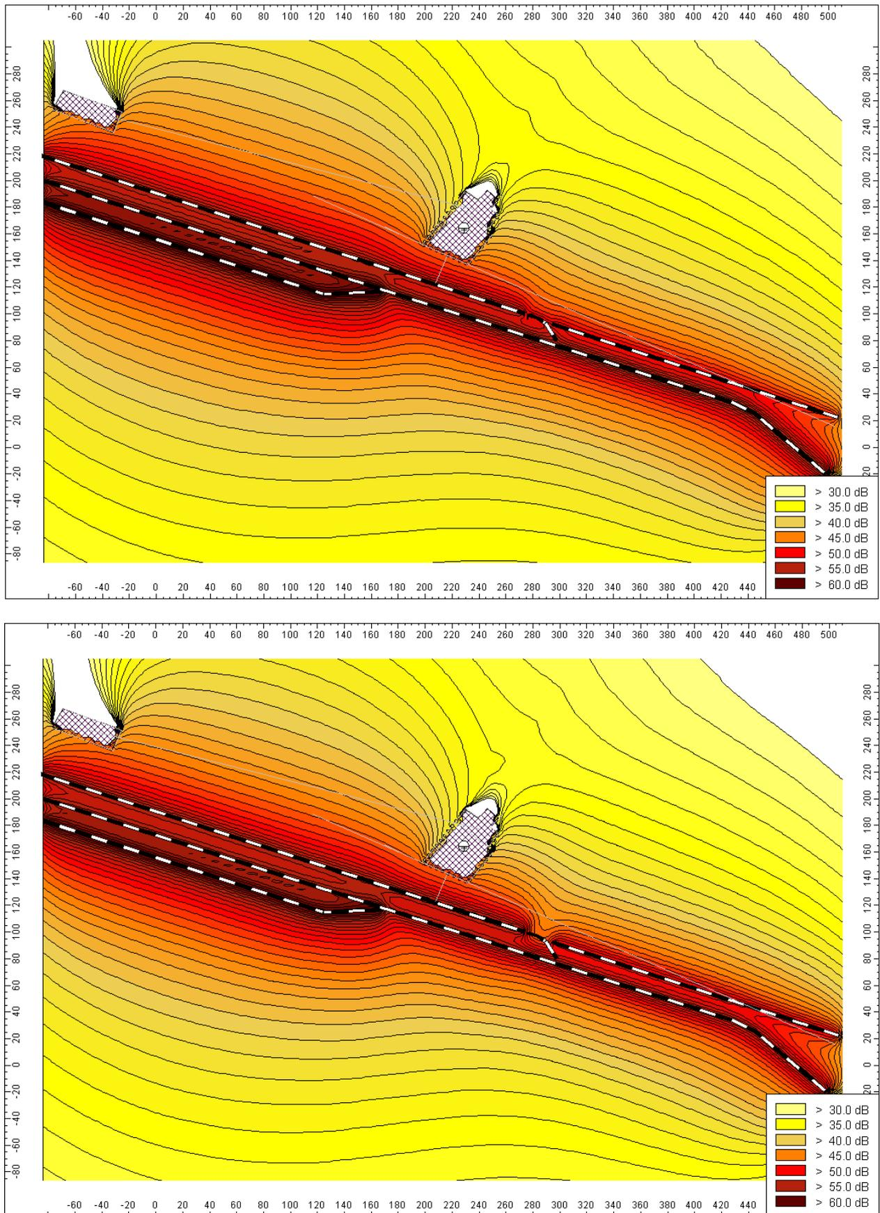
Fig. 5 A contour plot map of  $L_d$  (up) and  $L_n$  (down) of the acoustic emission due to the railway system working in the neighbour of Battipaglia station as seen from the detection building. Slight different are evidenced between the two pattern of emission.
