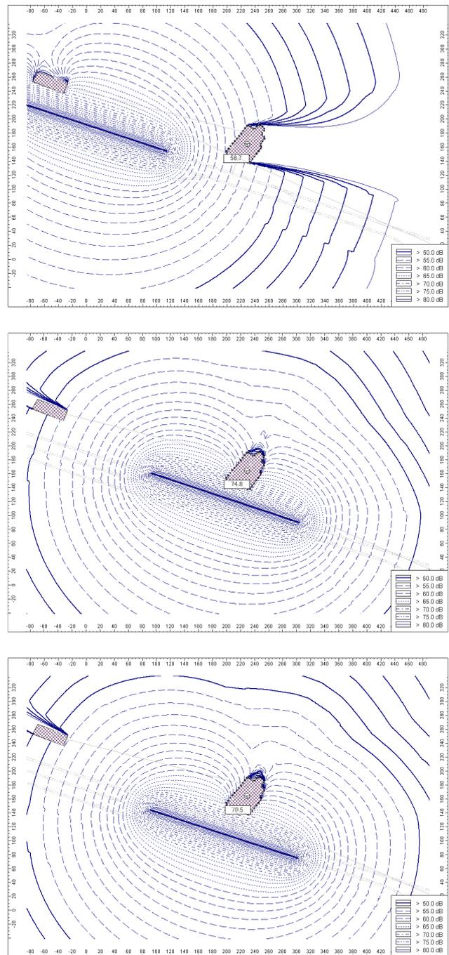
Fig.8 Simulation of train transit by means of a linear source. Left column: (top) a 120 dBA train transiting at the station level, (middle) a train with the same emission power in front of the detection building, (down) the same source placed on the intermediate railway.
