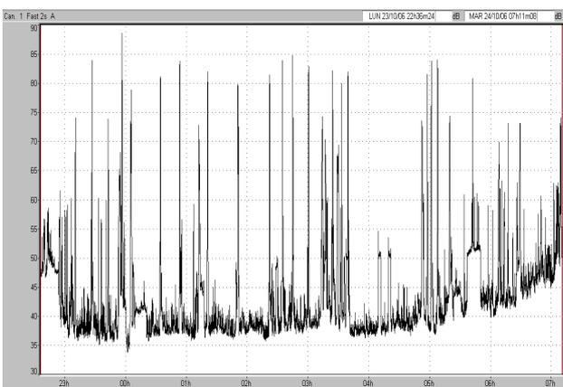
Fig. 3. Time history ( $L_{FastA}$  [dBA] vs  $t$  [s]) of whole acquisition period with *dBTrait*
