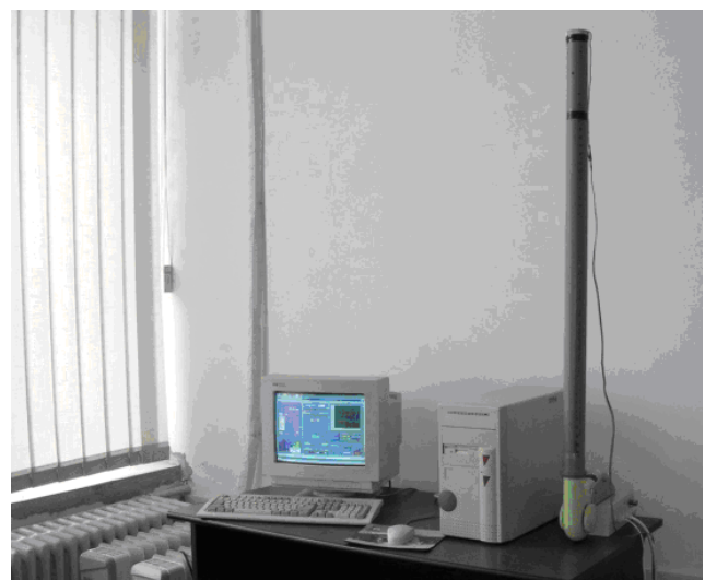
Fig. 7 Laboratory experimental nonlinear installation for positioning a ball in a vertical tube with a longitudinal opening
