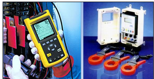
Fig. 8. Power quality analyzers
