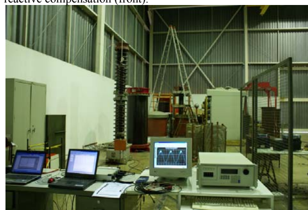
Fig. 23 - Calibration test setup at the lab – Power quality analyzer at left and arbitrary waveform generator, at right.
