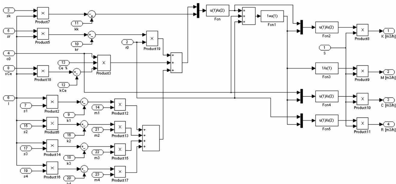
Fig.2. Block diagram for calculation of the material flows from the charge
