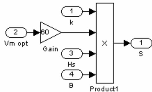
Fig.6. Block diagram for calculation of the charge flow
