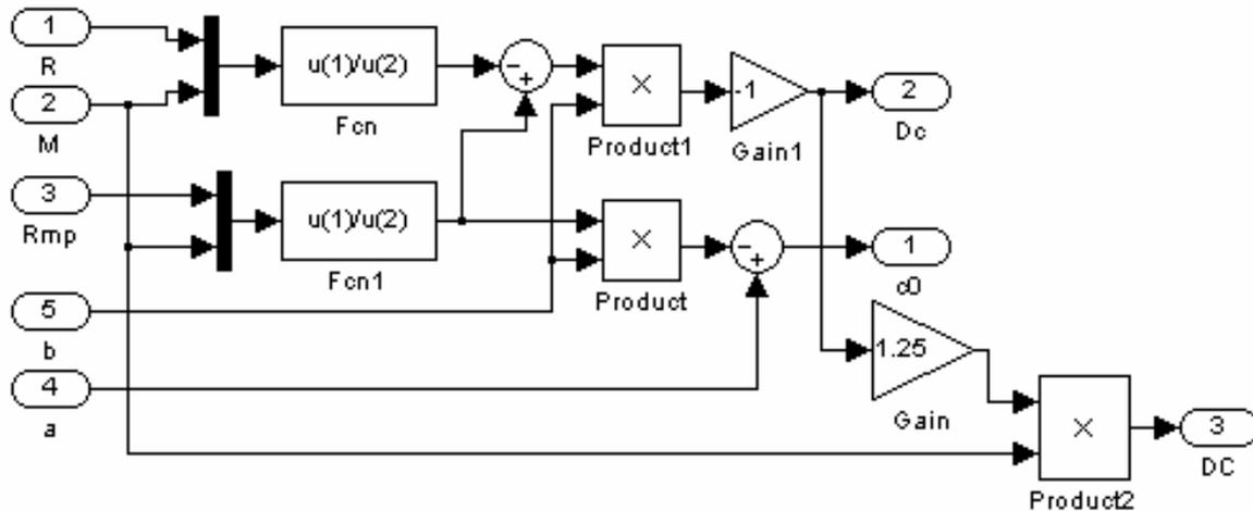
Fig.5. Block diagram for calculation of the coke content's variation from the charge
