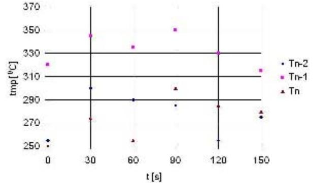
Fig.11. The temperature values for the three suction chambers, in time, for the simulation from fig.12
