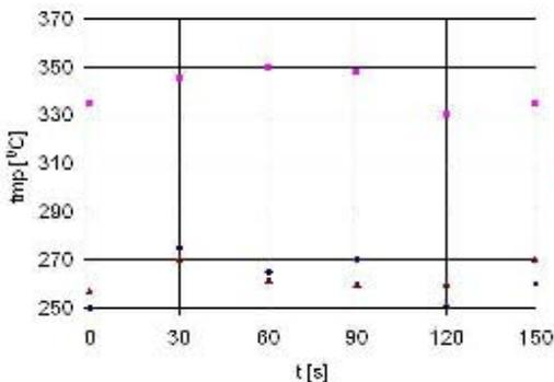
Fig.9. The temperature values for the three suction chambers, in time, for the simulation from fig.10
