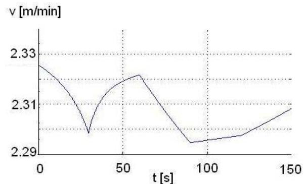
Fig.14. Variation of the sintering machine's optimal speed – case 4
