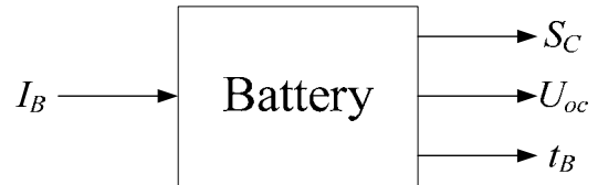
Fig.6 Input and outputs of the battery model
