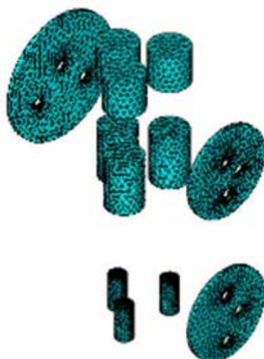
Fig.4(b) the three dimensional mesh of epoxy resin
