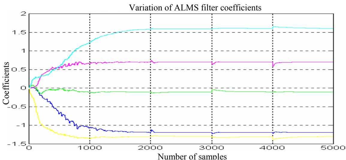
Figure 8. Variation of ALMS filter coefficients, SHARF algorithm, direct form.
