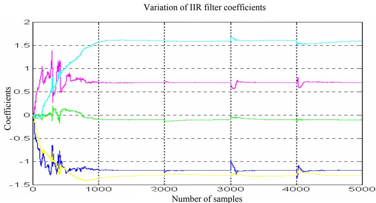
Figure 13. Variation of IIR filter coefficients, Steiglitz-McBride algorithm, direct form..
