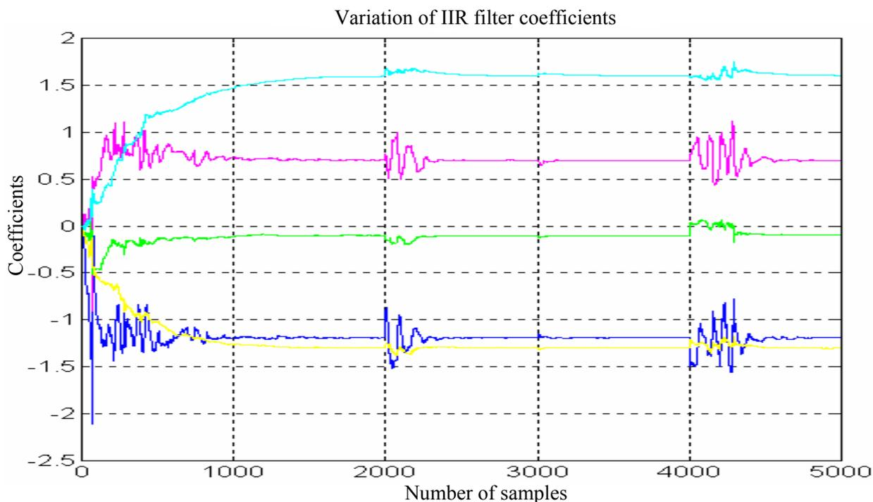
Figure 14. Variation of IIR filter coefficients, Steiglitz-McBride algorithm, lattice form.
