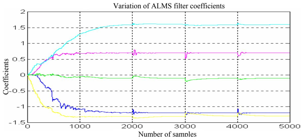
Figure 11. Variation of ALMS filter coefficients, SHARF algorithm, lattice form.
