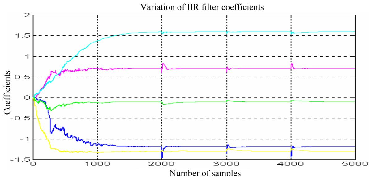
Figure 10. Variation of IIR filter coefficients, SHARF algorithm, lattice form.
