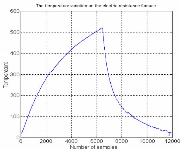
Fig. 17. The filtered measured temperature variation.
