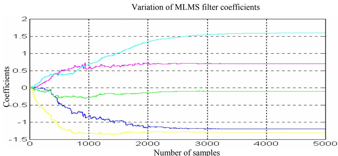
Figure 9. Variation of MLMS filter coefficients, SHARF algorithm, direct form.
