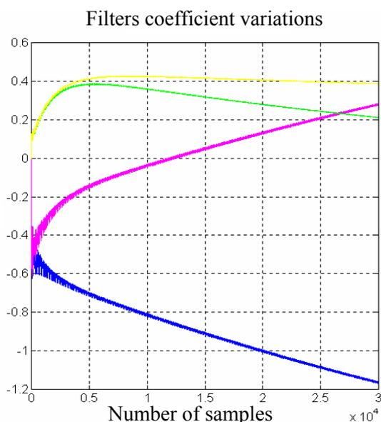
Fig. 18. Filters coefficients variations for  $\mu = 0,001$ .
