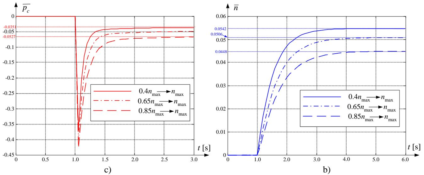
Fig. 9. System's step response ( $\bar{p}_c$  and  $\bar{n}$ ) for other engine's operating regimes
