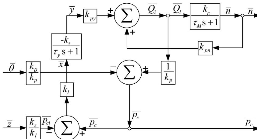
Fig. 4. System's simplified block diagram with transfer functions
