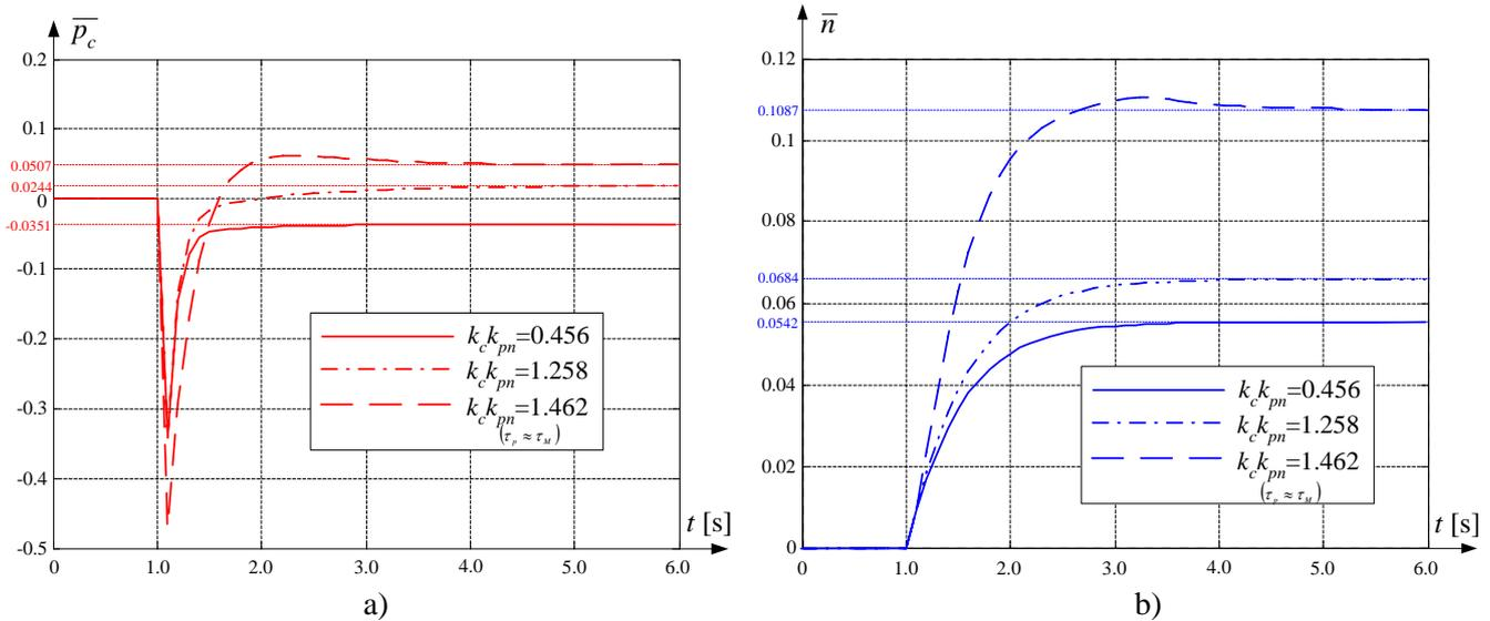
Fig. 10. System step response for maximum acceleration of jet engines having different  $k_c k_{pn}$  values
