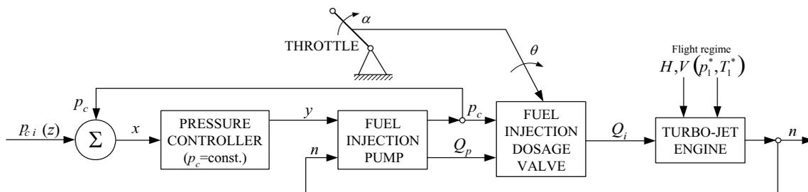
Fig. 2. System's functional block diagram
