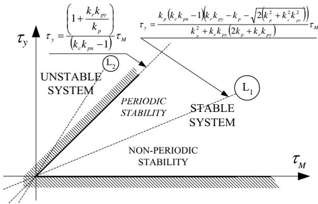
Fig. 7. System's stability domains (for  $k_c k_{pn} > 1$ )
