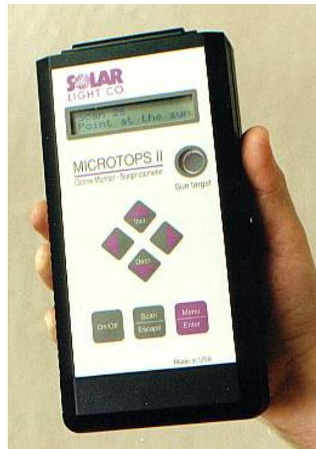
Fig. 12: MICROTOPS II portable SPM
