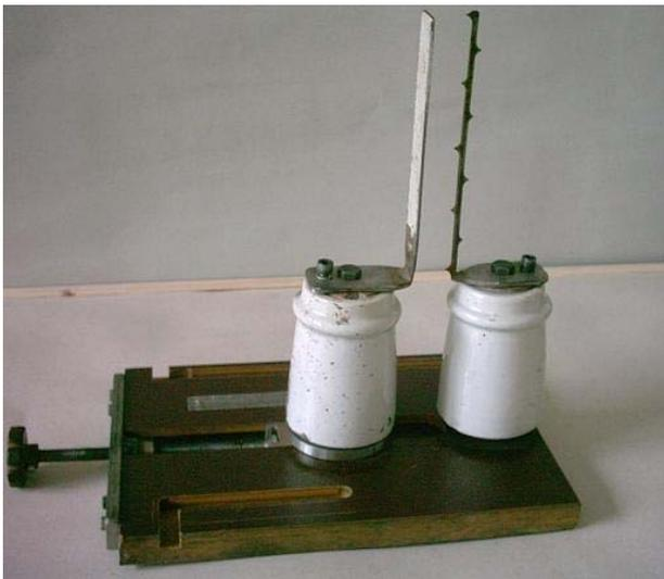
Fig.3. Electrostatic discharge system used in experiments
