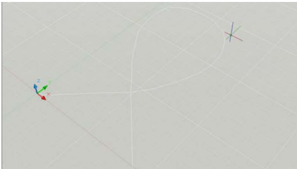
Fig. 14 1.5 foot trajectory sketched with 1270 lines
