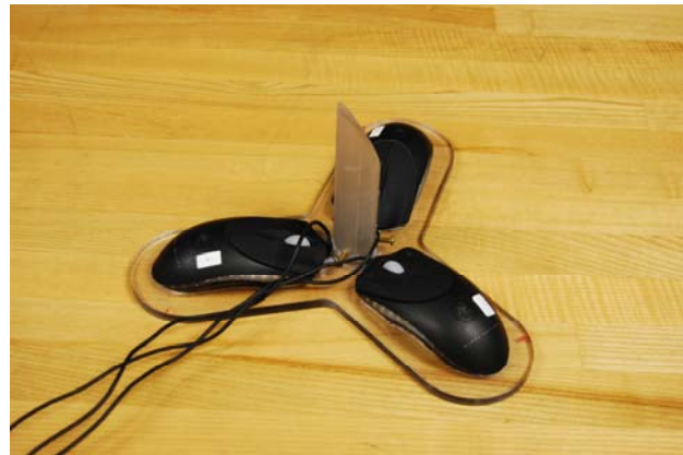
Fig 9. Three-mouse positioning jig
