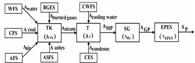
Fig.1 Block diagram for parametric reliability analysis of a turbogenerator
