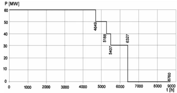
Fig.6 Power availability of turbogenerator obtain by the means of reliability block diagram
