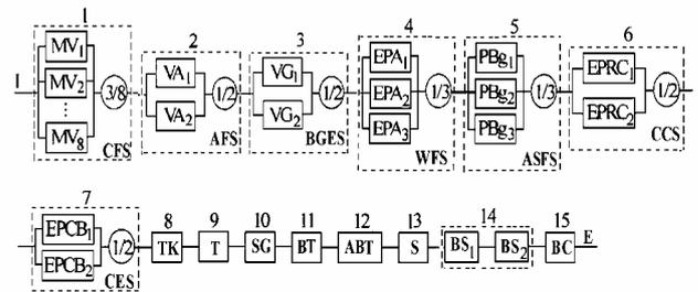
Fig. 5 Block diagram for parametric reliability analysis of a tubogenerator for 50% availability level
