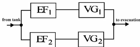
Fig.3 Block reliability diagram of subsystem
