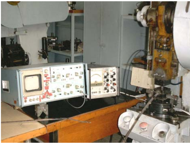
Fig. 22 The device used in punching of a sample
