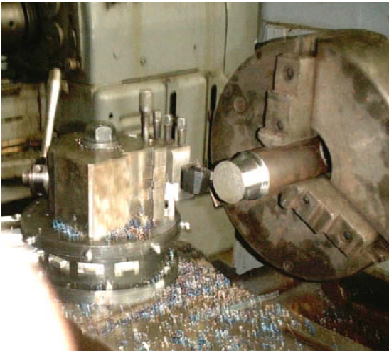
Fig. 18 The device used in exterior cylindrical turning of a sample
