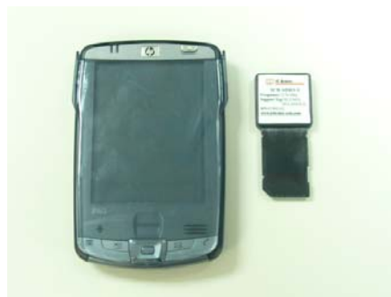
Fig.8. The handheld device, PDA, and the RFID reader (SD type of interface).
