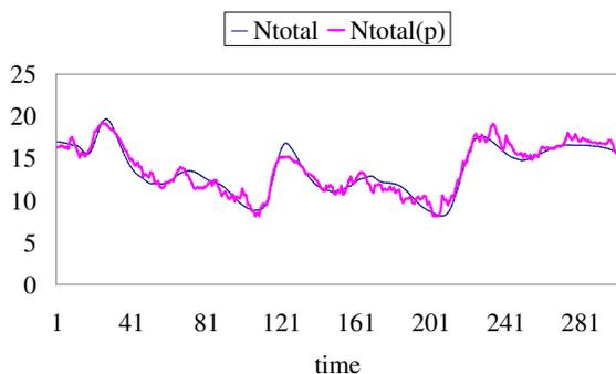
Figure 4: Ntotal real rain data versus predicted rain data based on a Kalman filter with genetic algorithm variable selection for NN1
