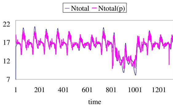
Figure 3: Ntotal real data versus predicted data based on a Kalman filter with genetic algorithm variable selection for NN2
