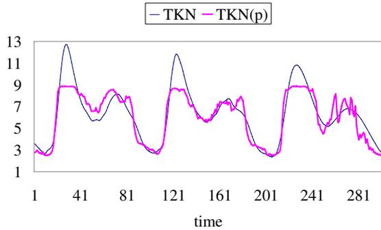
Figure 9: TKN real rain data versus predicted rain data based on a Kalman filter with genetic algorithm variable selection for NN1
