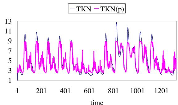
Figure 8: TKN real data versus predicted data by means a Kalman filter with genetic algorithm variable selection for NN1
