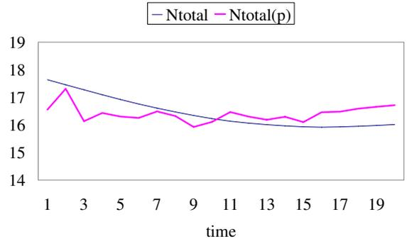
Figure 7: Ntotal: real 20 new data versus predicted 20 new data based on a Kalman filter with genetic algorithm variable selection for NN2
