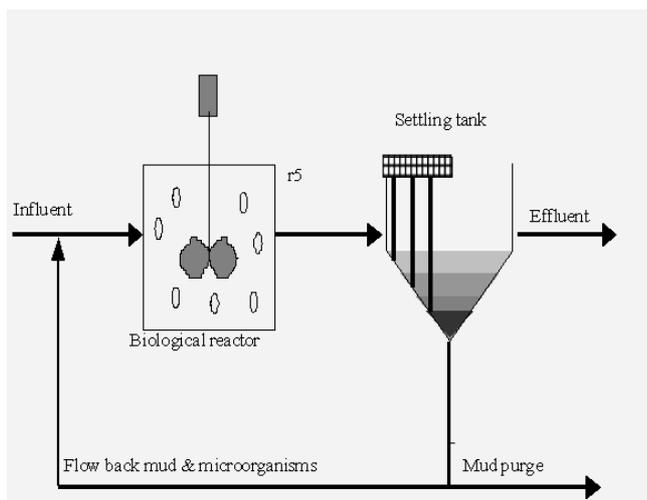
Figure 1: Schematic WWTP design
