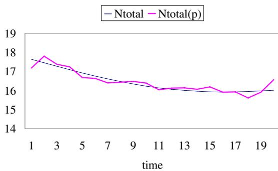
Figure 6: Ntotal: real 20 new data versus predicted 20 new data based on a Kalman filter with genetic algorithm variable selection for NN1
