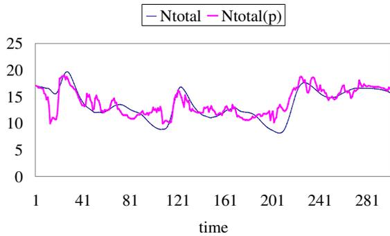
Figure 5: Ntotal real rain data versus predicted rain data based on a Kalman filter with genetic algorithm variable selection for NN2
