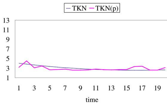
Figure 10: TKN: real 20 new data versus predicted 20 new data based on a Kalman filter with genetic algorithm variable selection for NN1
