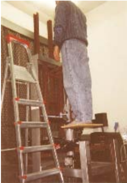
Fig. 15. Subjective method to verify the behavior of the human organism to vibrations
