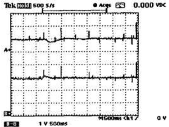
Fig.26 Waveform of Rotor Flux and Speed When Off-loading
