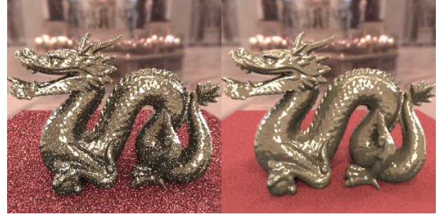
Fig.2: Dragon model in an indoor HDR EM. Left: Importance sampling from BDRF, 200 samples/pixel. Right: Bidirectional importance sampling.
