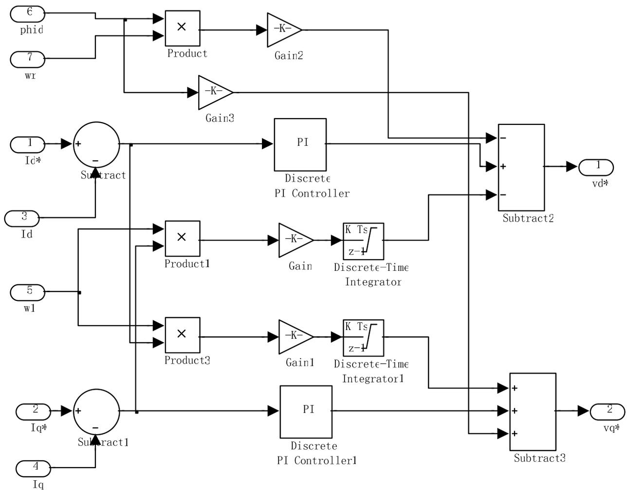
Fig.4 Current Internal-Model Controller
