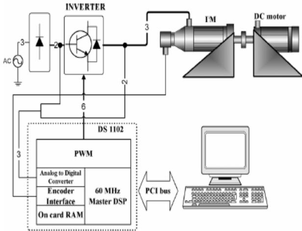
Fig. 11. Experimental setup for the asynchronous motor drive
