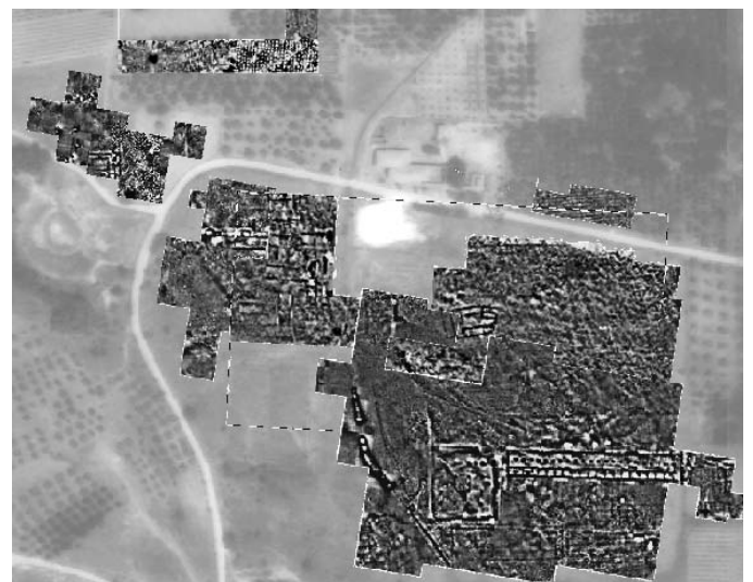
Fig. 2. The integrated results of the magnetic survey in the area of Sikyon. Magnetic data were collected through 3 different seasons employing a Bardington GRAD 601 and a Geoscan Research FM256 fluxgate gradiometer, using a 0.5m sampling strategy.
